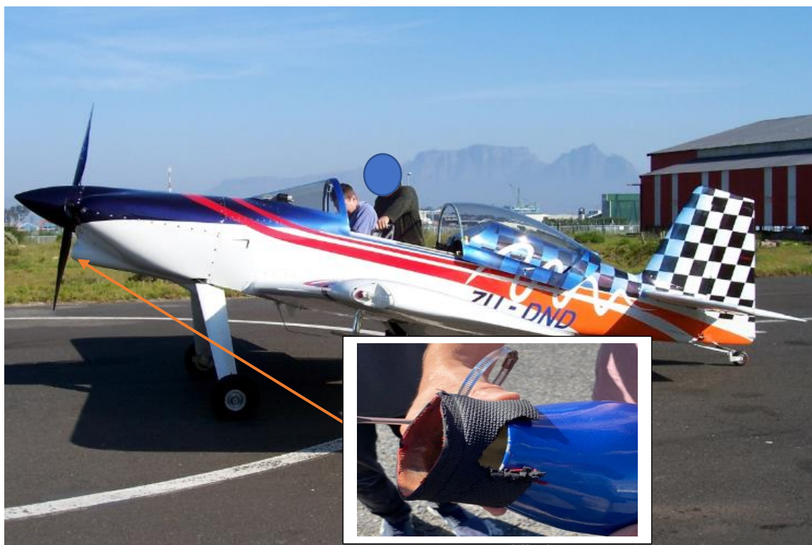
Figure 1: The baffle seal of the engine induction filter housing. (Source: Pilot)
