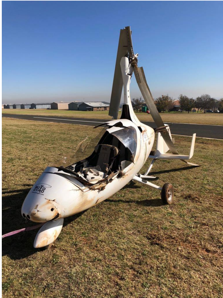
Figure 5: The damage to the autogyro due to the high-speed blade flap
