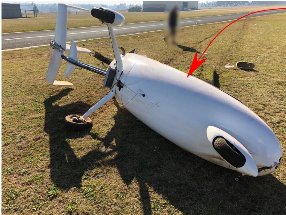
Figure 4: The arrow indicates the path that the autogyro slid after the high-speed blade flap.
