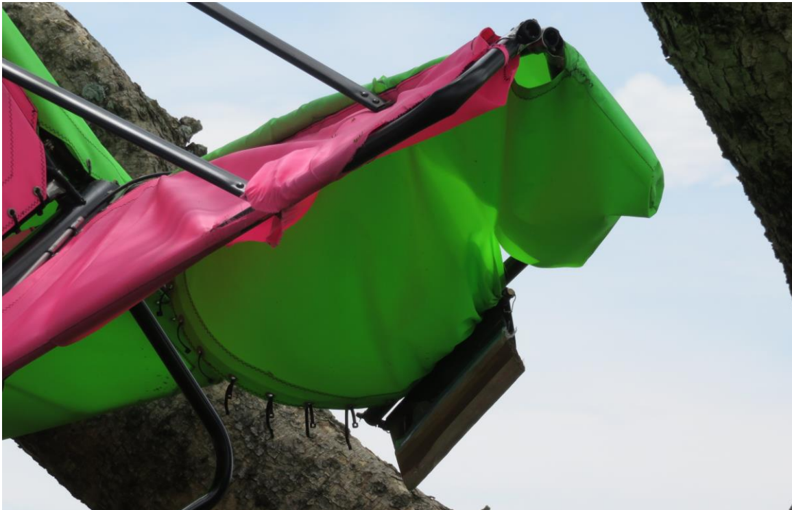
Figure 8: Damage to the empennage area, and the unapproved trim tab modification
