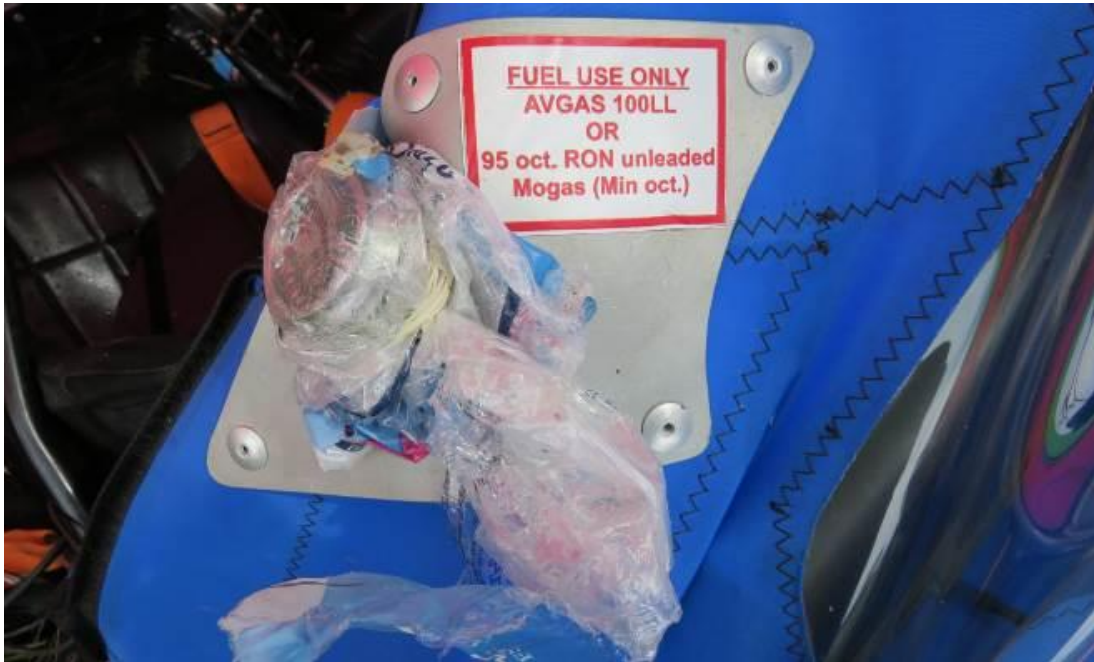
Figure 9: Plastic bag covering in place of the fuel cap
