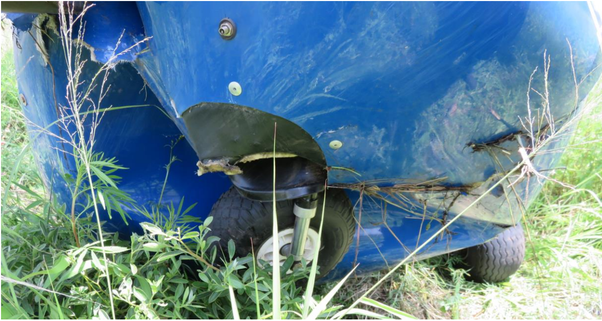
Figure 7: Collapse nose gear due to excessive impact forces
