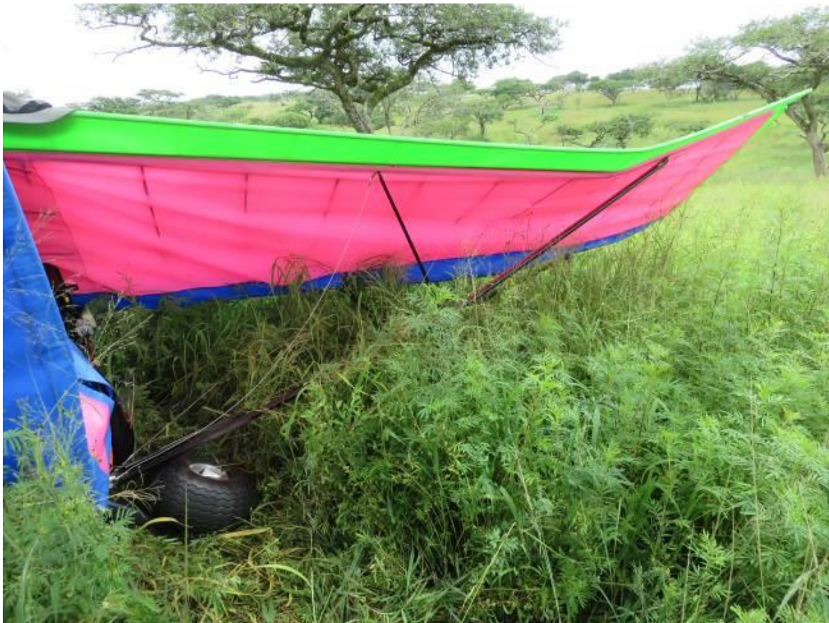
Figure 6: Distortion to the right wing and the collapsed right main gear
