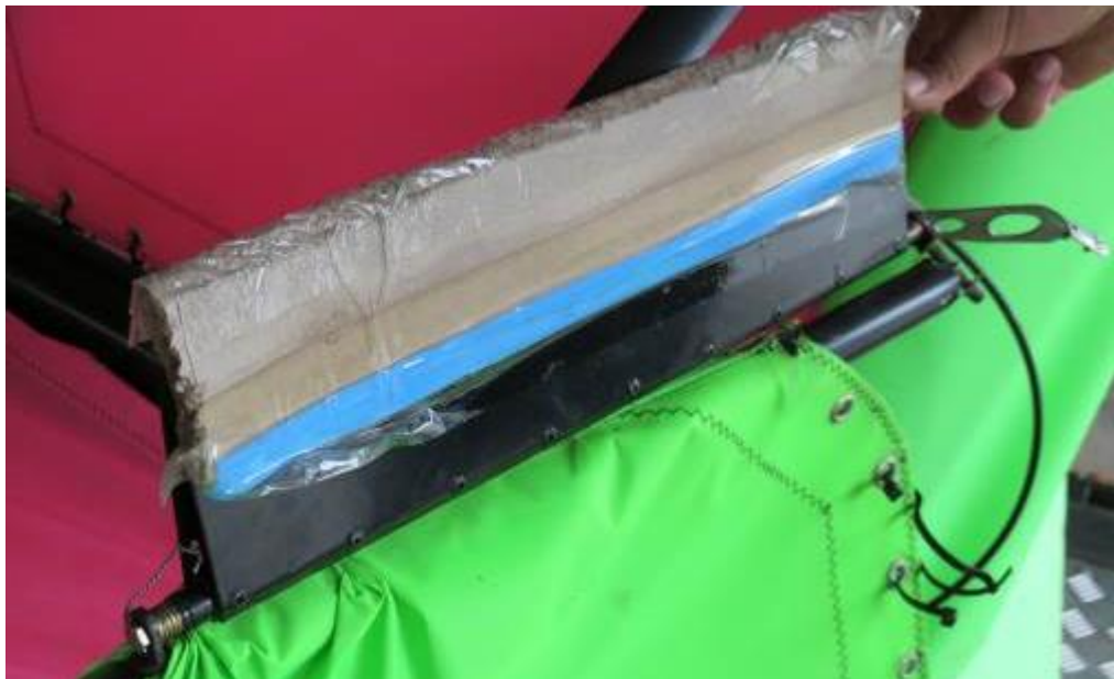
Figure 13: The elevator trim tab modification as it was found
