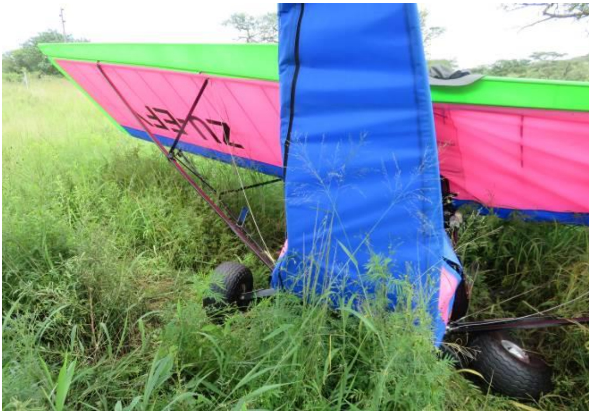
Figure 12: High tail attitude due to the distorted fuselage
