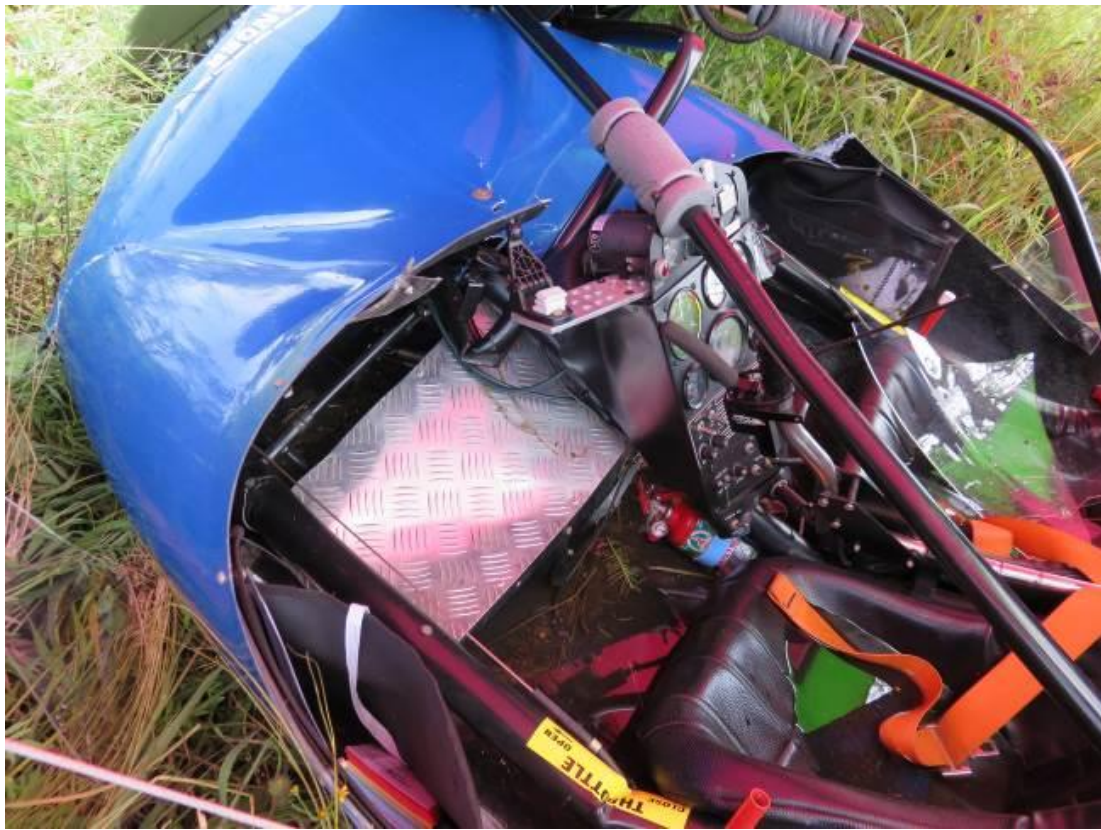
Figure 5: Damage to the controls and cabin area. The Plexiglas window completely shattered and the fibre glass area around the pilot's legs collapsed due to the impact and fuselage distortion.
