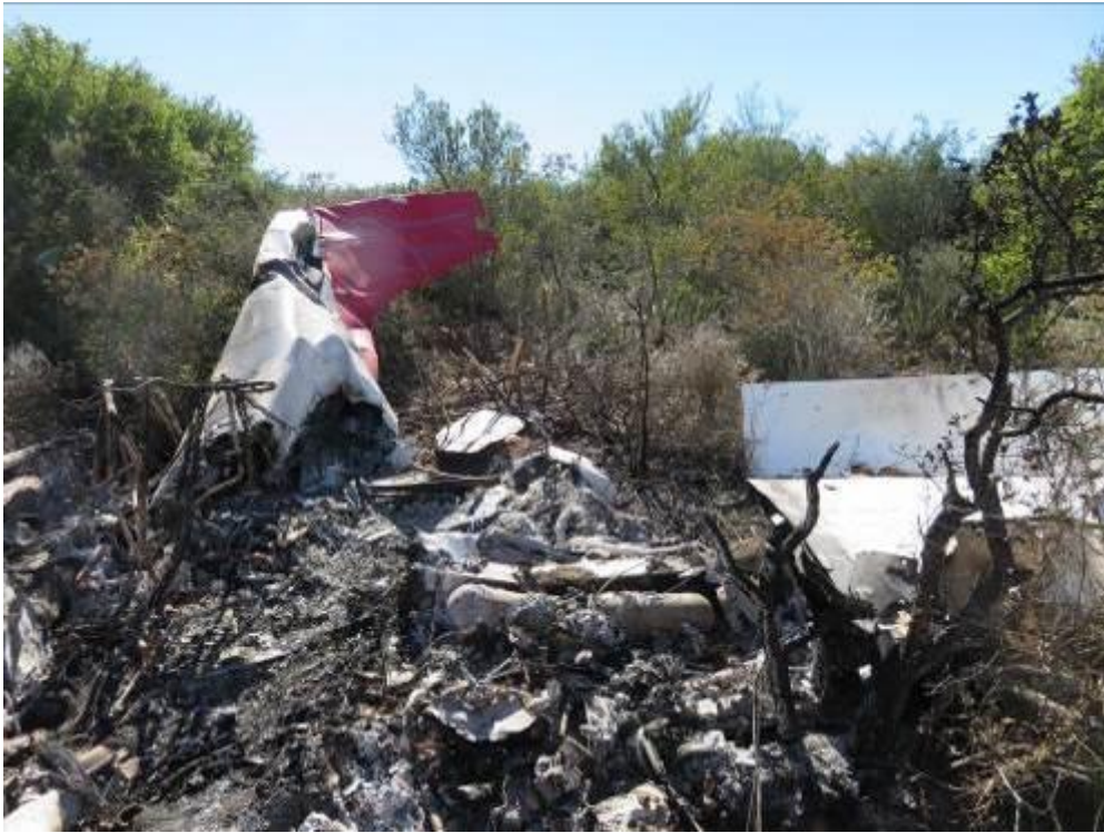
Figure 17: The cockpit/cabin area was consumed by post-impact fire
