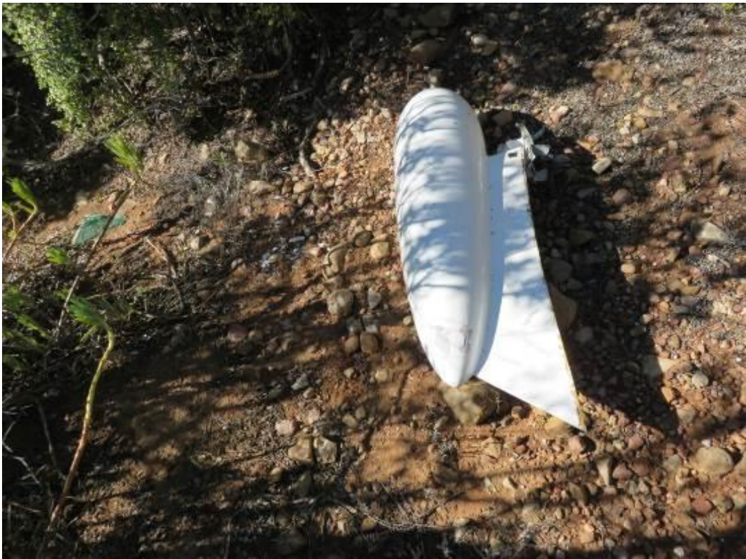
Figure 15: The Stormscope antenna that was mounted underneath the right wing
