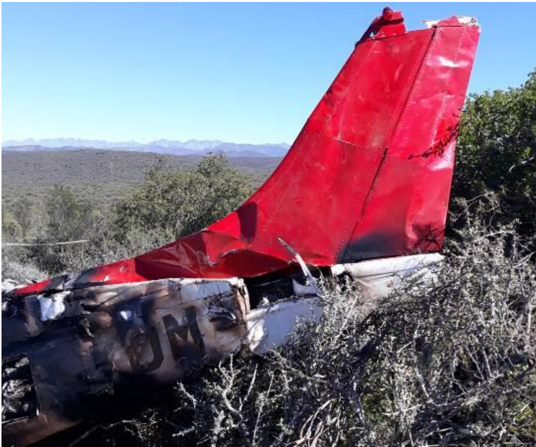
Figure 11: A view of the empennage (left-hand side) with the horizontal stabiliser and elevator missing
