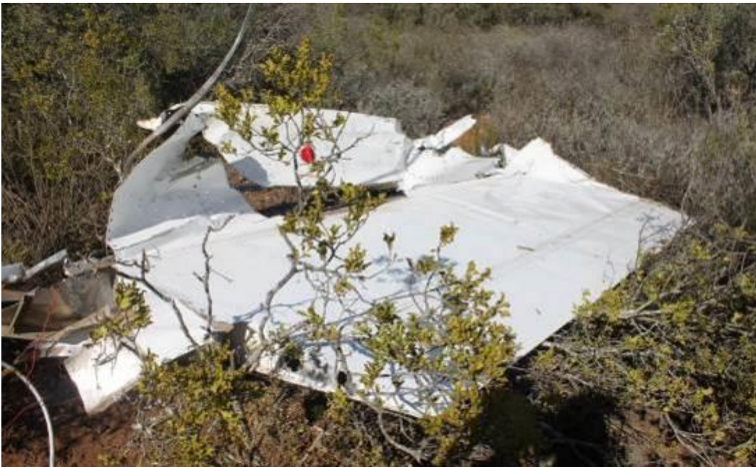
Figure 12: A major part of the left wing with the flap attached and in the up position
