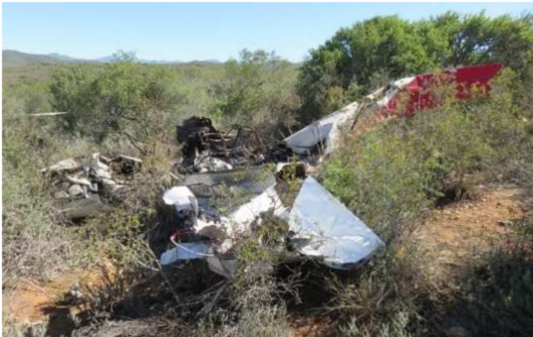
Figure 3: The main wreckage as it came to rest in an inverted attitude
