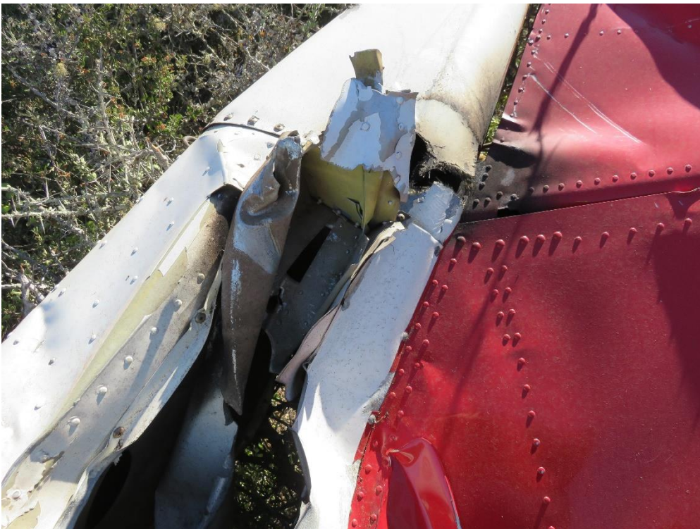
Figure 18: Deformation visible to the right aft fuselage where the horizontal tail plane was fitted
