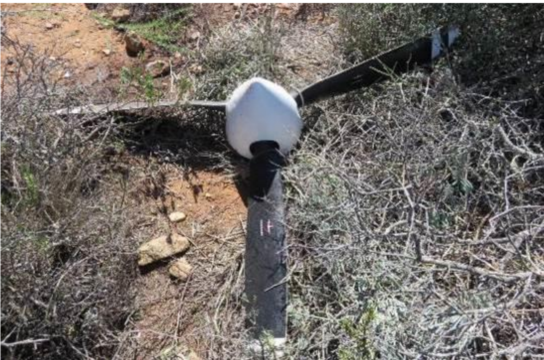
Figure 16: The propeller with the spinner still attached, displaying minor damage
