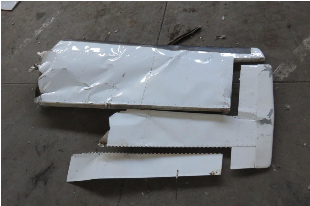
Figure 19: Some parts from the right horizontal tail plane that were recovered from the scene
