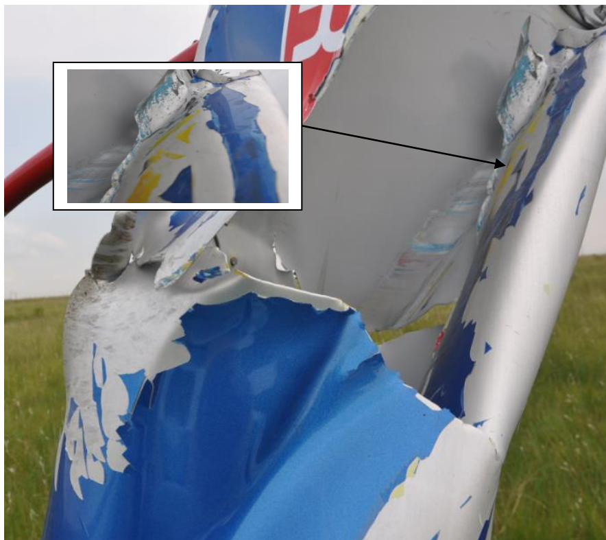
Figure 7: Yellow paint mark and blade imprint.
