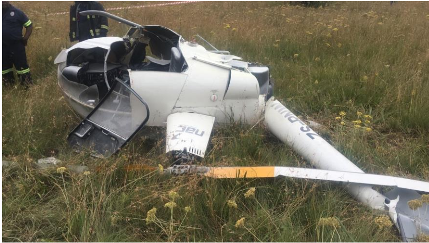
Figure 2: The rotor blades were mostly undamaged
