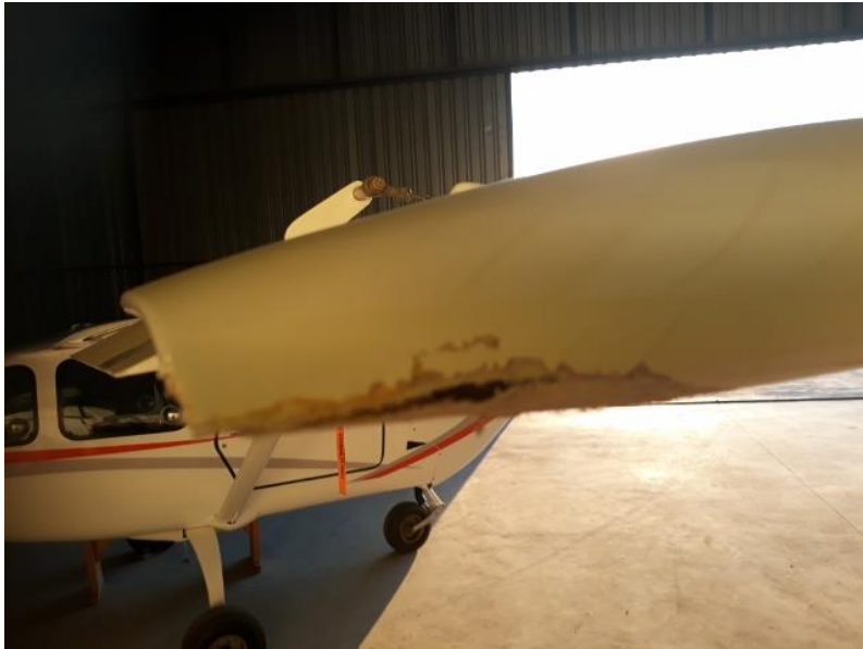
Figure 5: Shows damage on the right wing.
