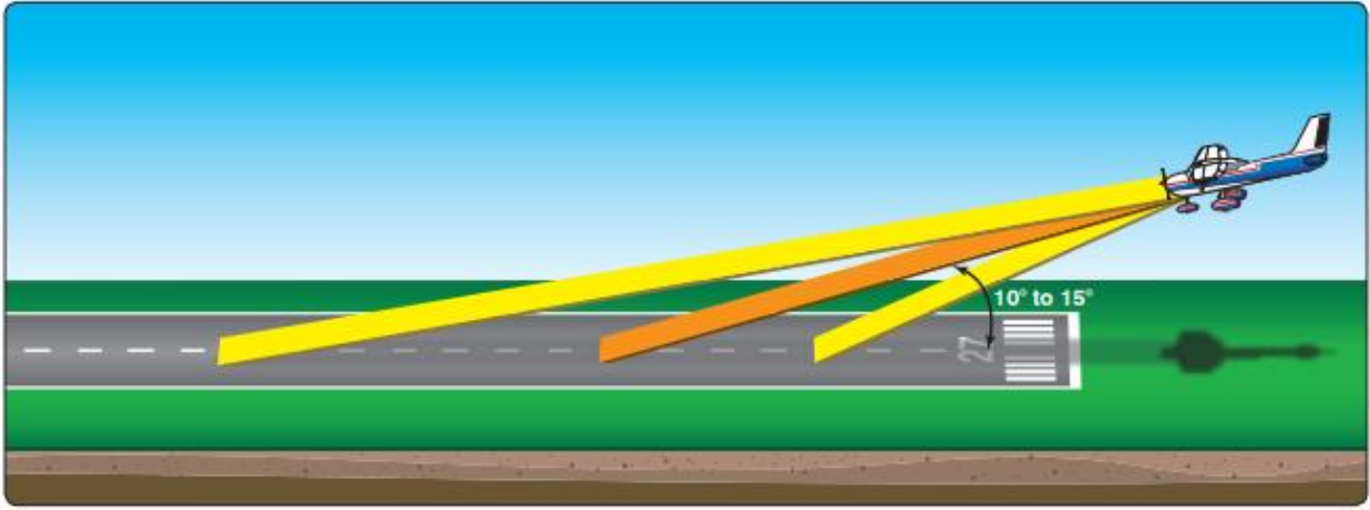
Figure 2: To obtain necessary visual cues, the pilot should look toward the runway at a shallow angle.
