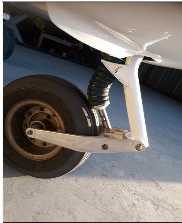
Figure 4: Shows damage on the nose gear.
