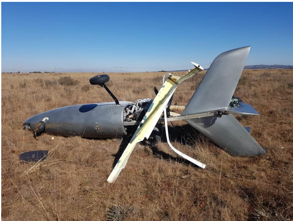
Figure 2: Damage to nose landing gear (courtesy of the owner of the aircraft)
