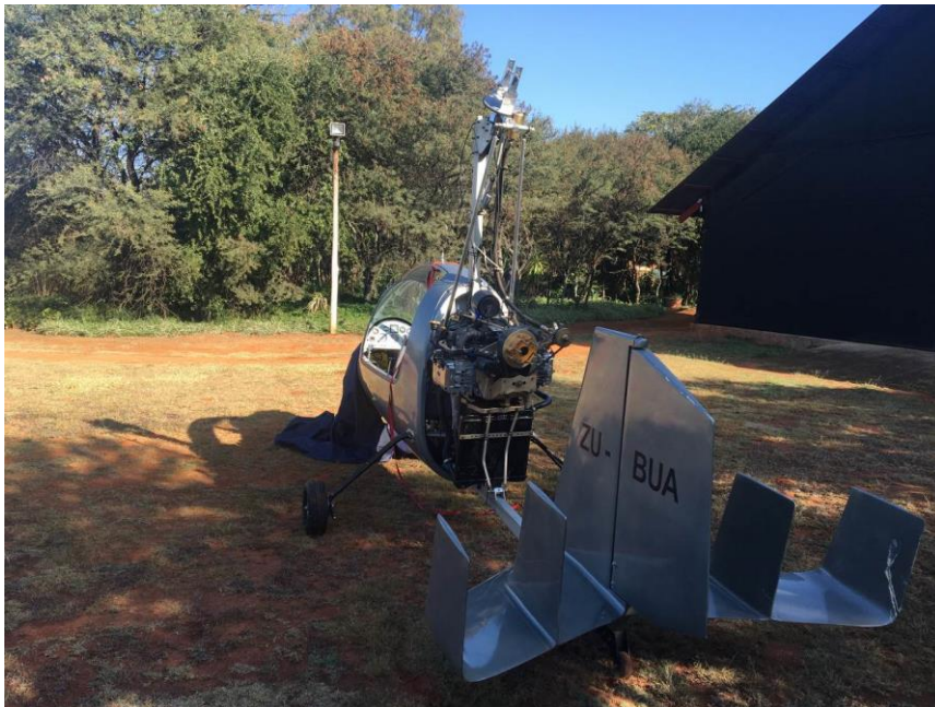
Figure 3: Shows damage to right-hand vertical stabiliser (picture taken after recovery)
