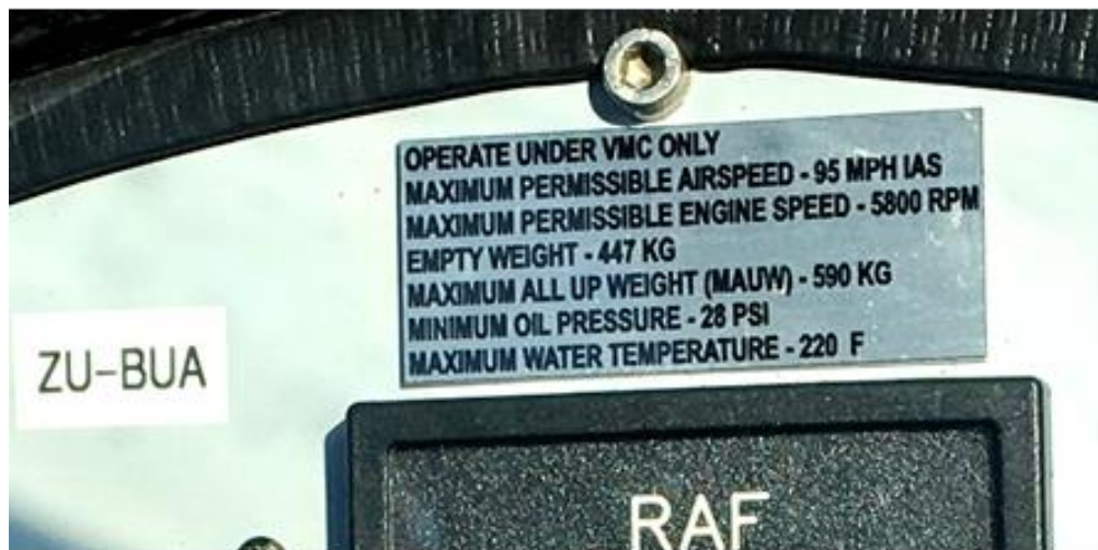
Figure 6: Shows a picture of the data plate on the instrument panel giving the MAUW as 590 kg
