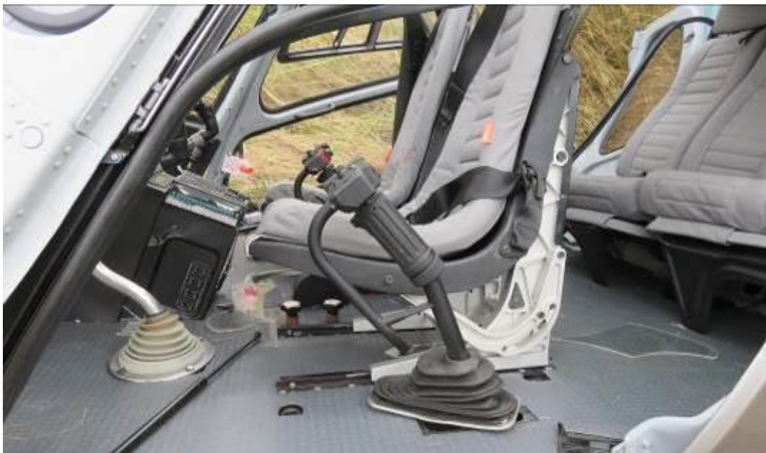
Figure 7: A side view from the left of the cockpit with the collective pitch levers in the full up position
