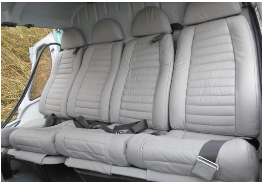
Figure 12: The four aft cabin seats, with the cabin structure that remained intact
