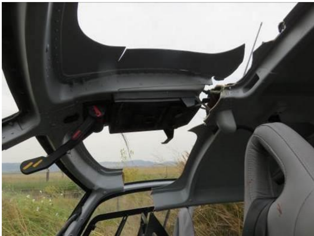
Figure 14: Inside view of the damaged roof structure, with the rotor brake/fuel shut-off quadrant visible
