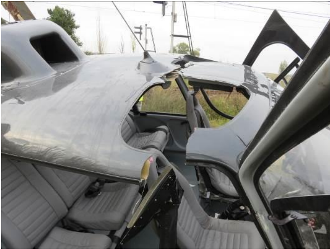
Figure 13: Failure of the roof structure
