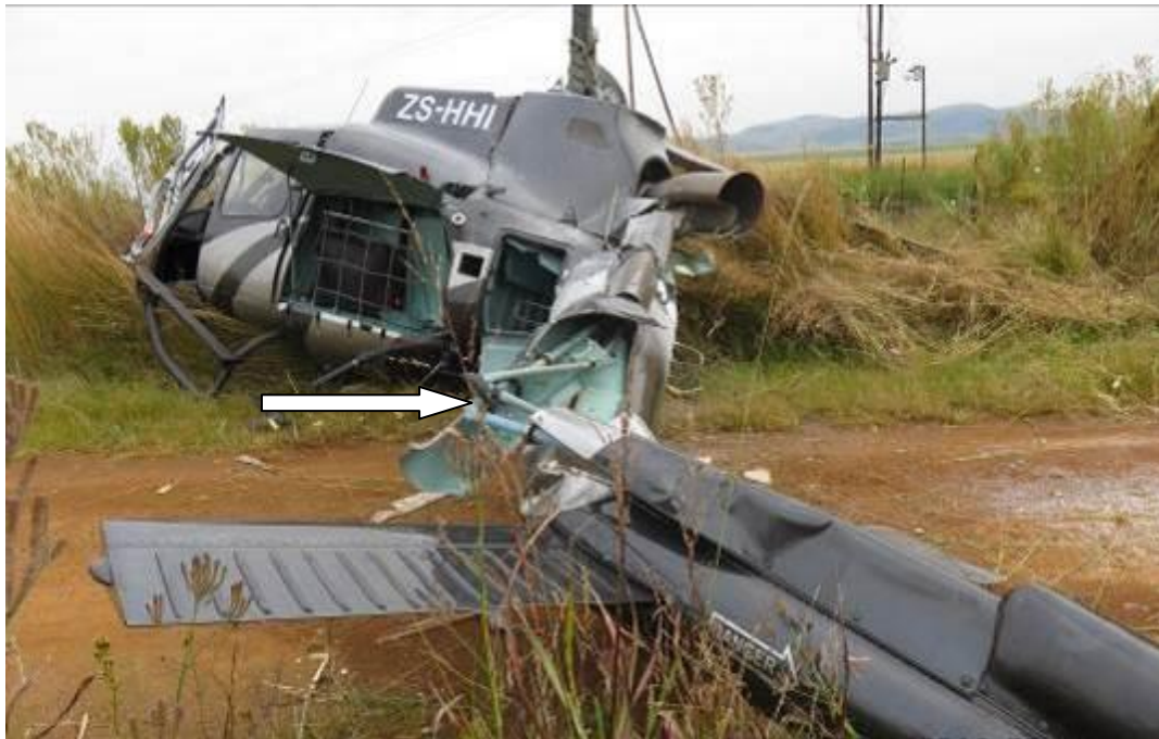
Figure 10: The tail rotor drive shaft and tail boom, having been struck by the main rotor blades
