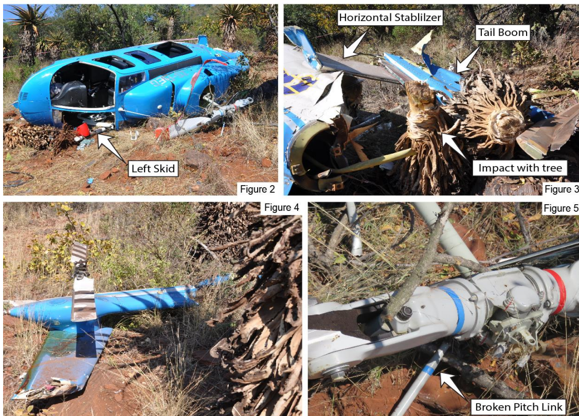
Figure 2: The wreckage as it lay on its port side on the broken left skid, Figure 3: Separation of the tail boom and fuselage resulting from impact with the tree., Figure 4: The separated tail rotor assembly. The tail rotor blades are still intact, but the strobe section impacted terrain and separated, Figure 5: The main rotor hub showing one broken pitch link. The other pitch link was broken off. (Figures 2, 3, 4 & 5 sourced from IIC)
