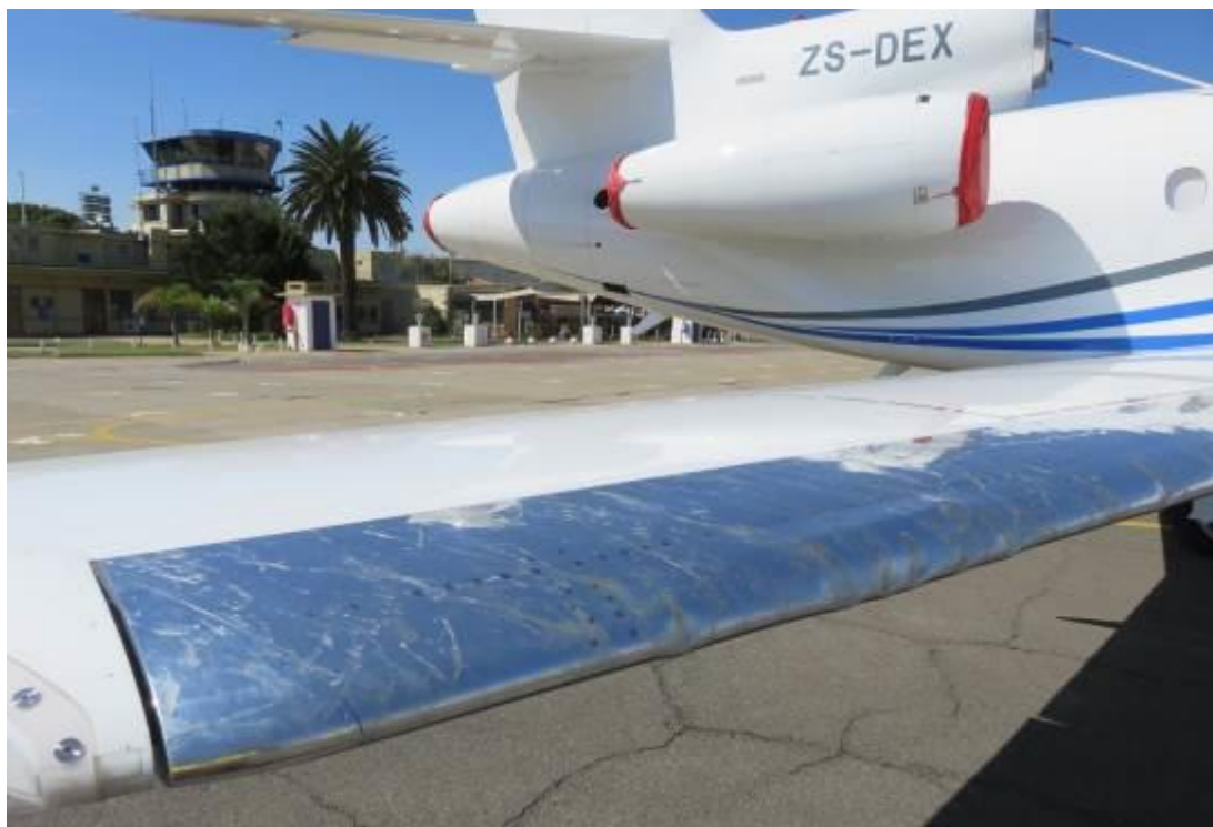
Figure 13: Damage to the right-wing slat, which was caused by vegetation (impact with trees)
