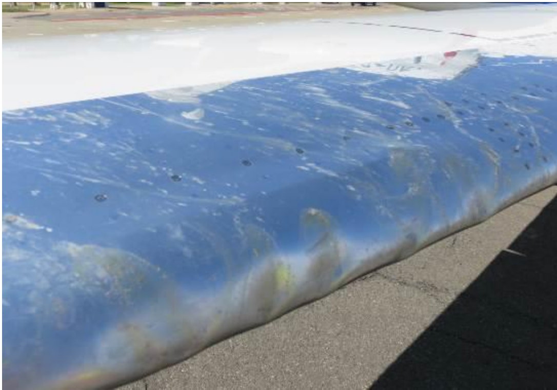
Figure 14: Closer view of the damage to the right-wing slat
