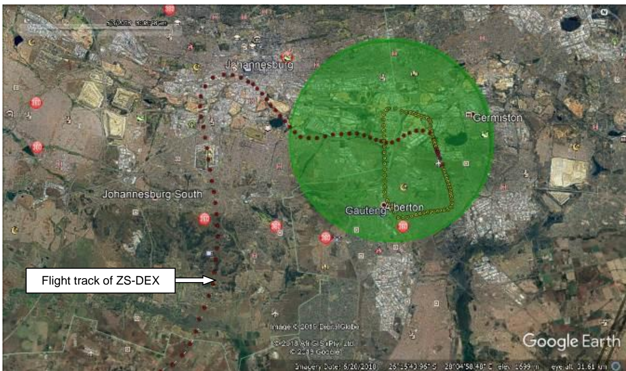
Figure 1: Overlay of the approach path that was flown by ZS-DEX (red dotted line)
