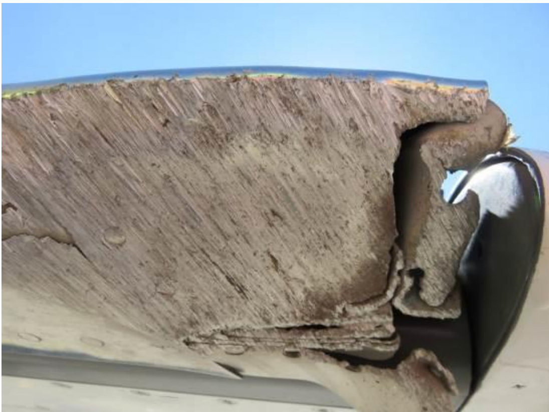
Figure 11: Damage to the left-wing leading edge slat, lower surface
