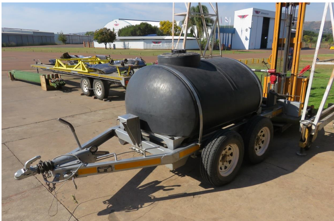
Figure 1: The fuel trailer/bowser that was used for refuelling the helicopter (photograph taken at Wonderboom Aerodrome (FAWB) by an Accident and Incident Investigation Division (AIID) investigator)
