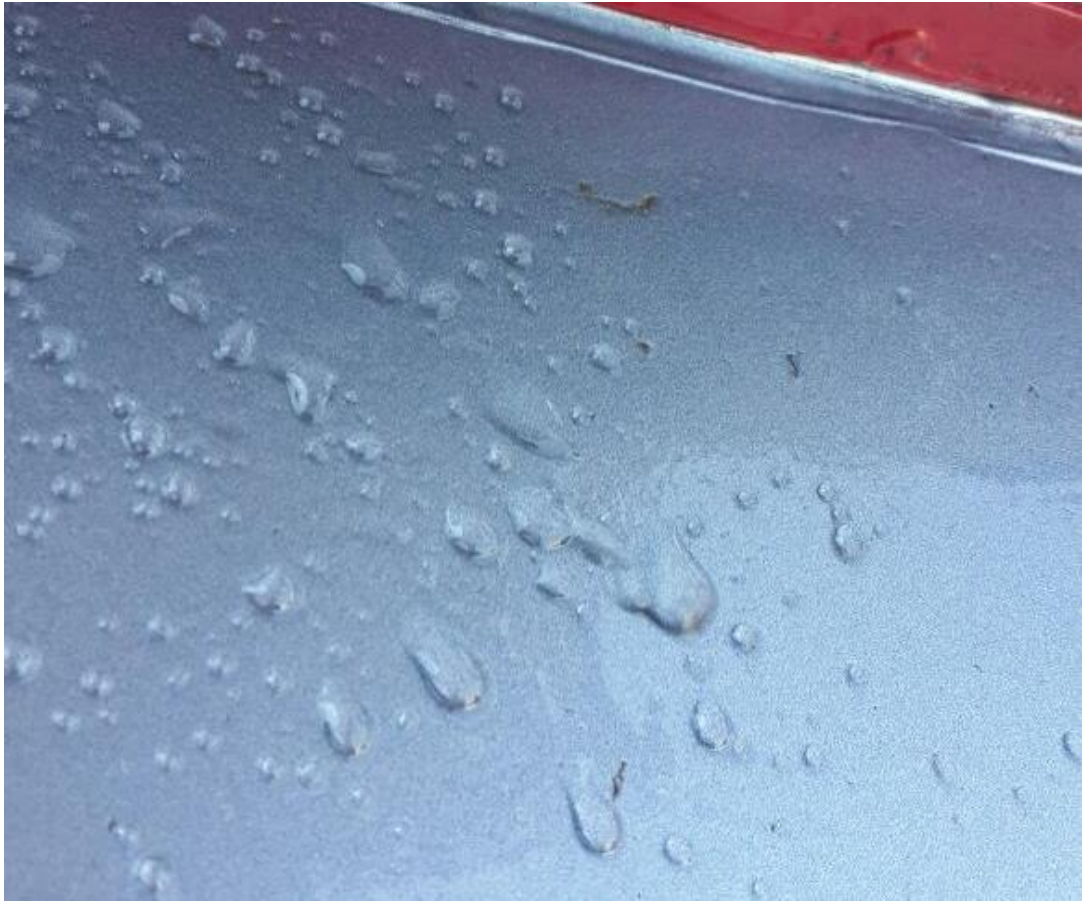
Figure 4: Water droplets from the FCU fuel filter following the removal of the filter unit
