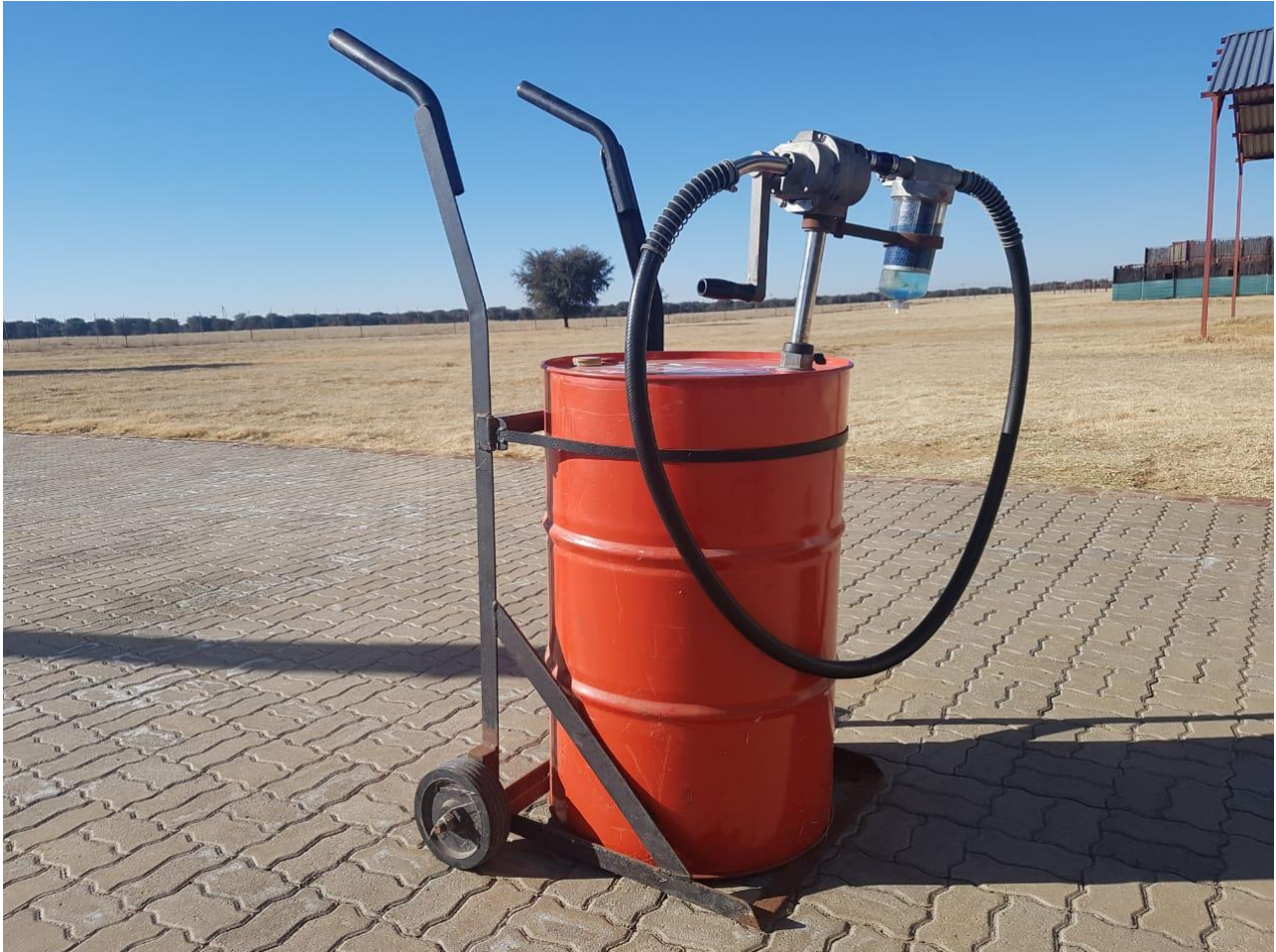
Figure 7: The drum mentioned in paragraph 1.4.2 which contained Avgas used to refuel ZS-RBJ (This photograph was obtained from the pilot / owner of the helicopter)
