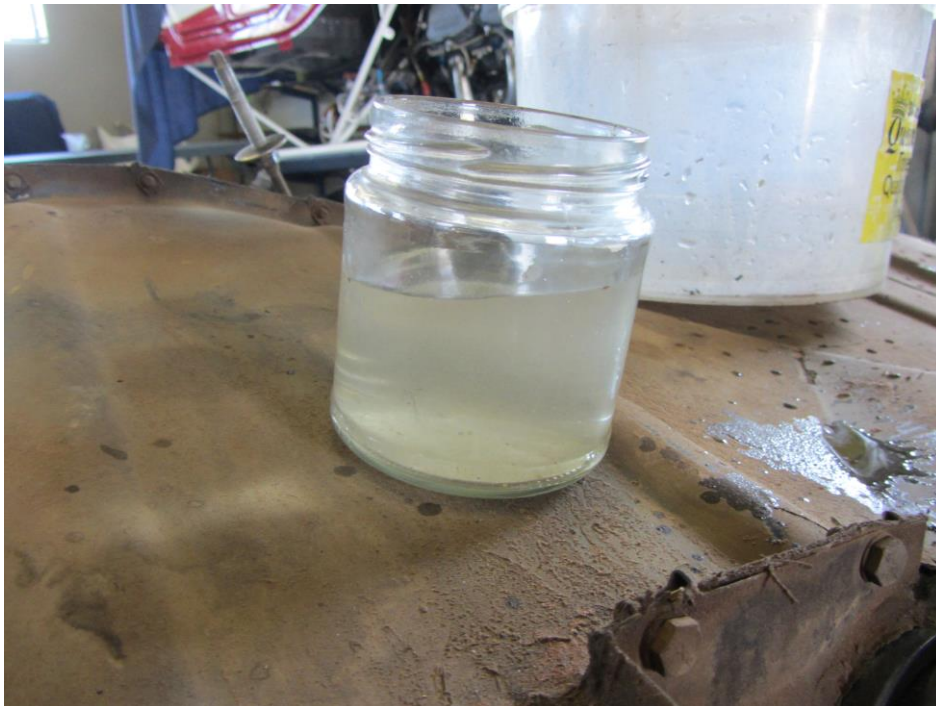
Figure 5: The glass container displaying water that was found in the fuel lines of ZS-RBJ.
