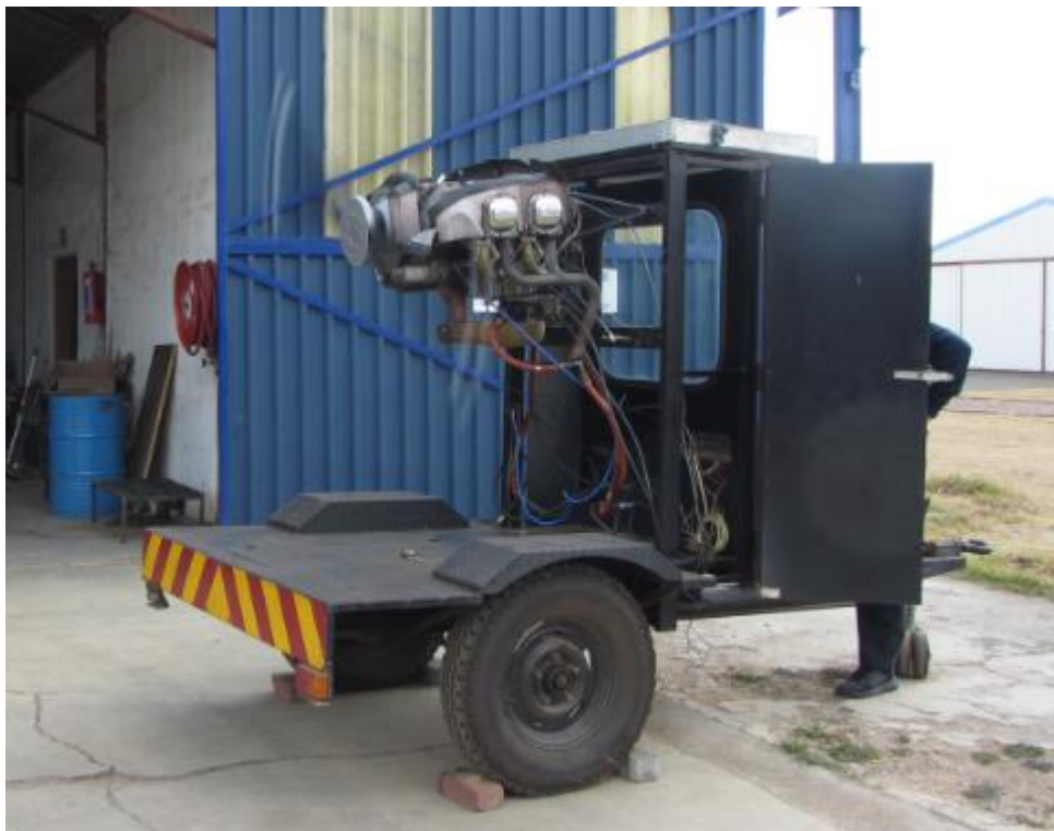
Figure 11: Engine on the test bench running at full throttle.
