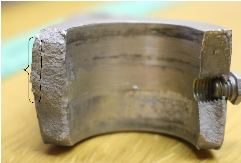
Figure 4: The side brace showing a fractured pivot point.
