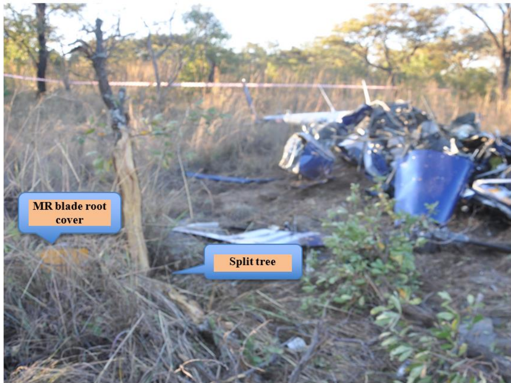
Figure 10: Image shows the split tree and a MR blade root cover.
