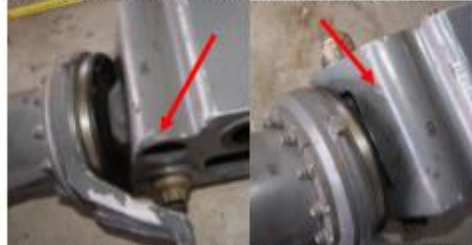
Photo 7: Impact damages to MR Hub assembly (digital)
