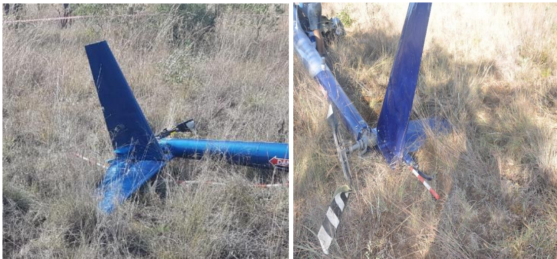
Figure 16 & 17: Images show broken tail rotor blade and a damaged horizontal stabiliser.
