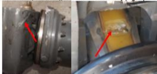
Photo 8: Impact damages to MR Hub assembly (digital)
