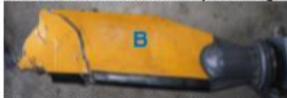
Photo 18: Blade B, Section 3, failure direction and position (digital)
