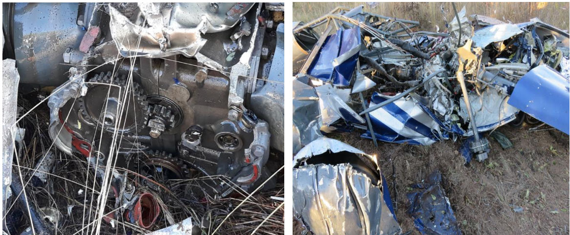
Figures 14 & 15: Images show damage to the engine and drive train.
