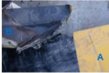
Photo 14: Blades A and B, impact scraping marks (digital)
