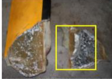
Photo 20: Blade B, Section 3, impact damages to honeycomb structure (digital)
