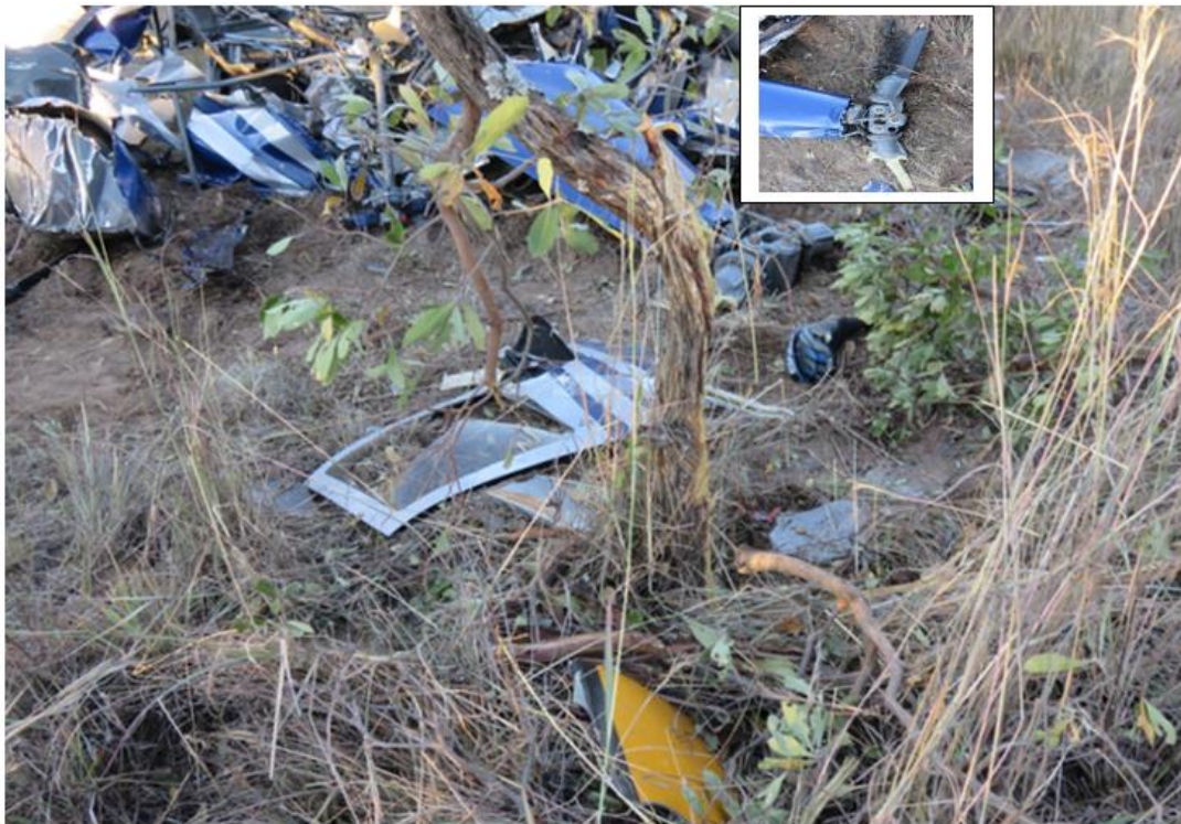
Figure 11: Shows the blade root still attached to the main rotor hub
