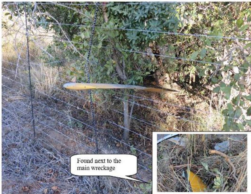
Figure 12: The MR blade as found at the accident site.
