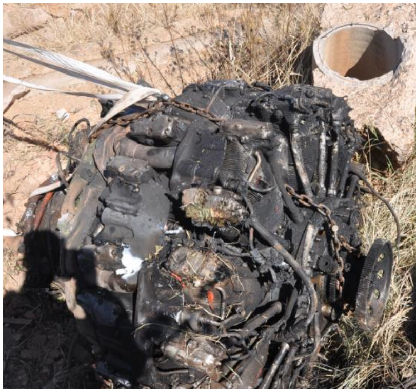
Figure 25: The right-hand engine as it came to rest with black soot indicating exposure to fire.
