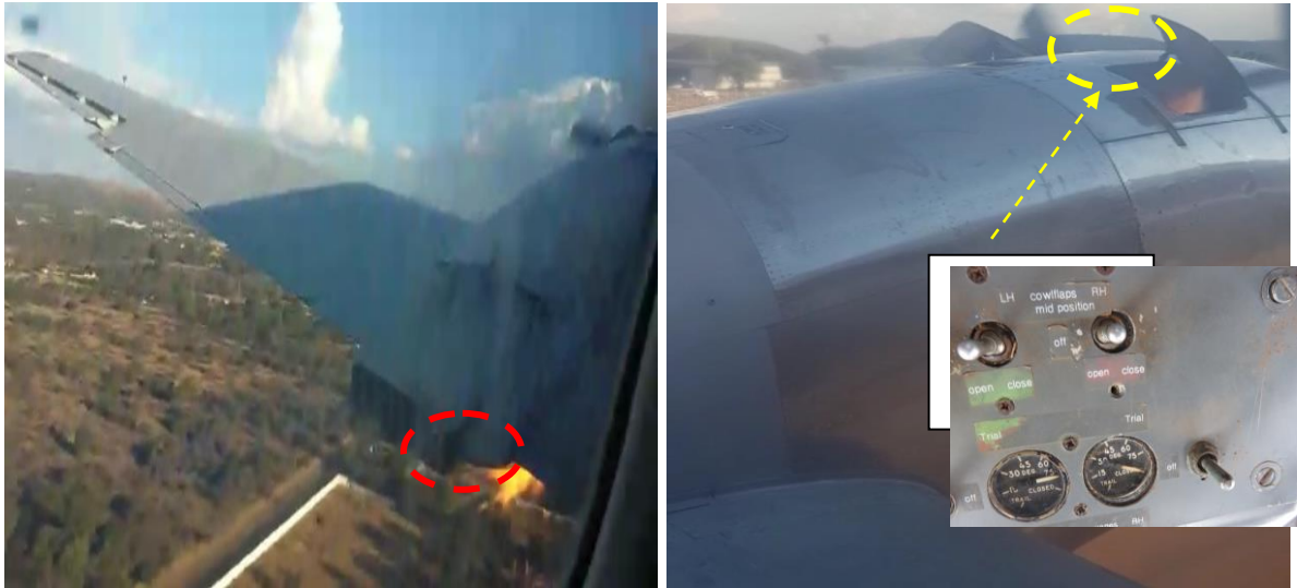
Figures 2/3: Images of the left wing and engine taken from the cabin. The image circled in red (left) shows the fire trailing underneath the left wing. The one circled in yellow (right) shows fire emanating from the left engine (No 1) compartment with the cowl flaps in the open position.
