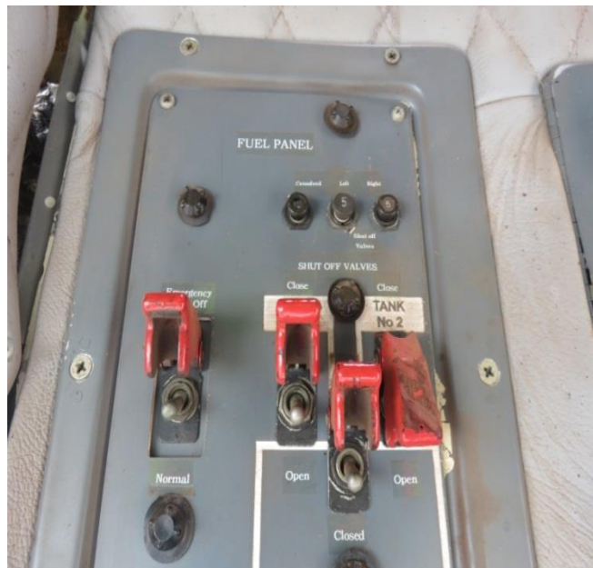
Figure 11: The fuel panel as it was recovered from the accident site.
