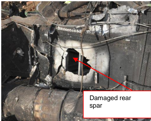
Figure 26/27: Images showing fire damage on the left-wing rear spar and pulley attachment brackets separated from the spar with its pulleys and the cables.
