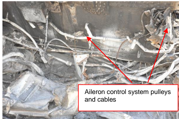
Figure 26/27: Images showing fire damage on the left-wing rear spar and pulley attachment brackets separated from the spar with its pulleys and the cables.
