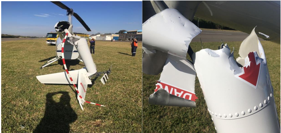
Figures 1 & 2: Damage to the tail boom
