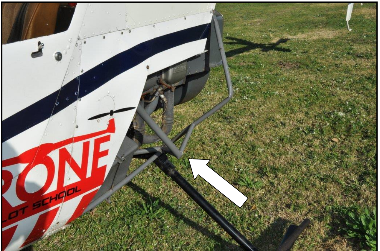
Figure 2: Damage to the rear left frame
