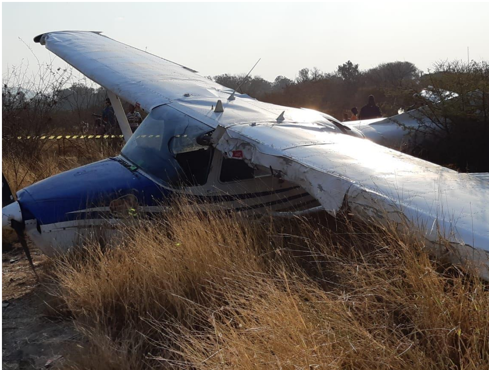
Figure 2: Damage sustained to the aircraft after the runway excursion
