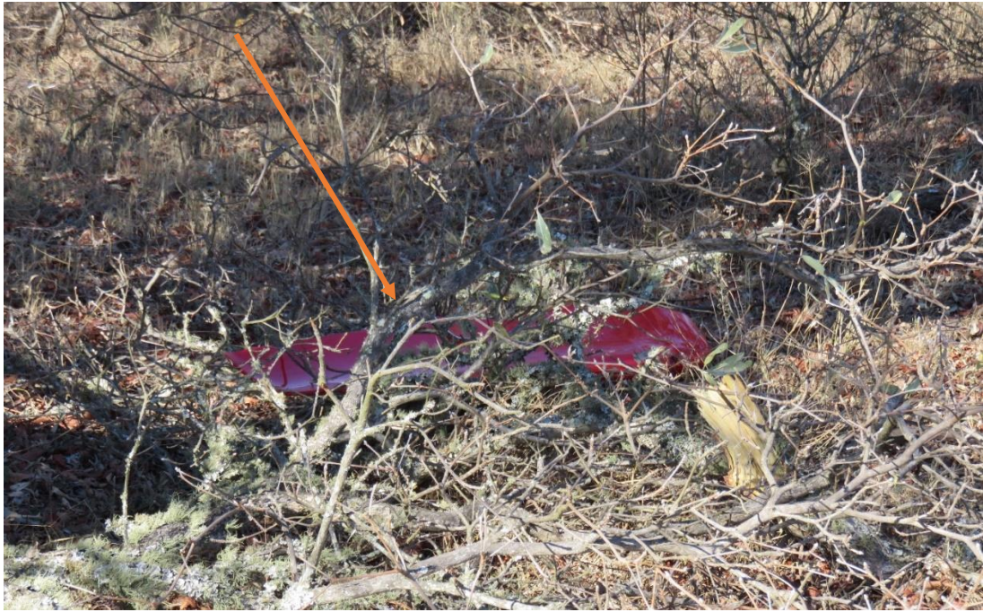
Figure 4: The arrow shows the broken wingtip lying among debris from the tree
