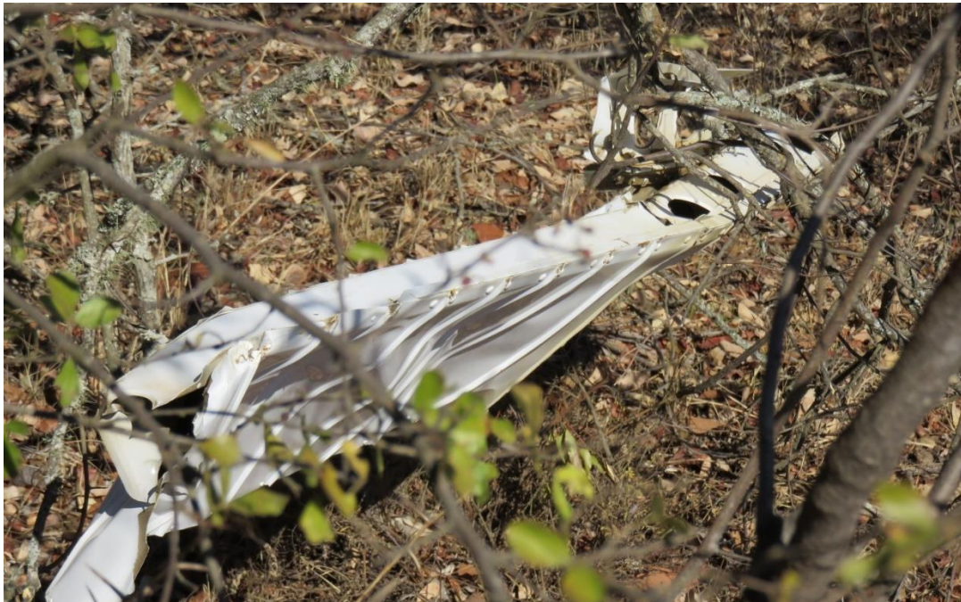
Figure 5: The broken portion of the aileron
