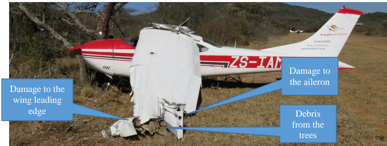
Figure 6: Damage sustained to the left wing
