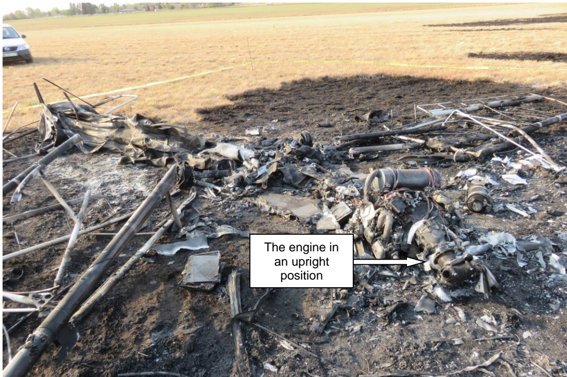
Figure 11: The engine was found in an upright position
