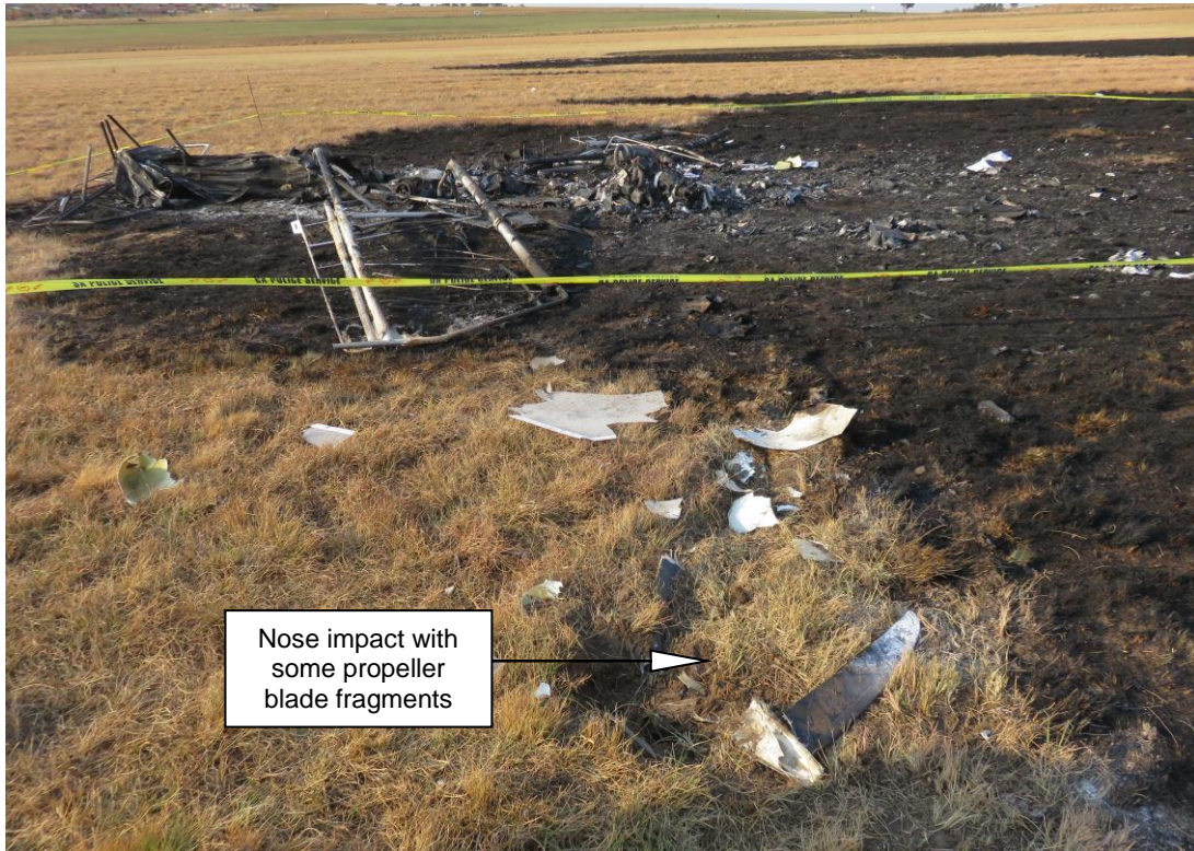
Figure 9: Nose impact markings with propeller blade fragments visible
