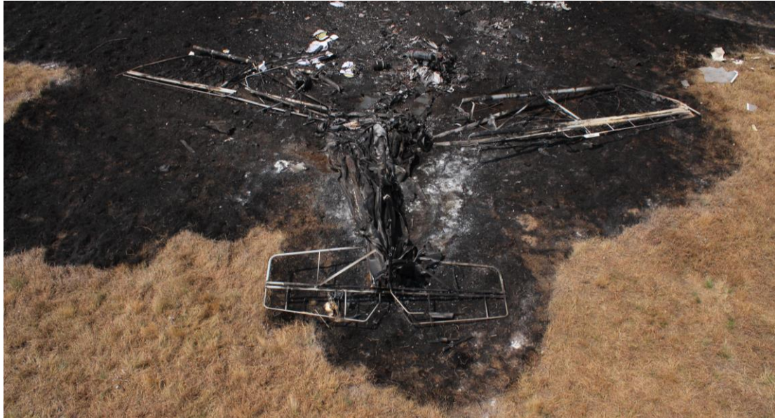
Figure 1: The wreckage was consumed by the post impact fire
