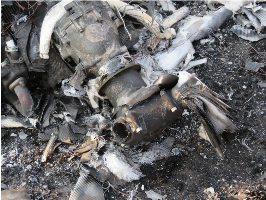
Figure 12: A closer view of the engine gearbox and the propeller flange assembly
