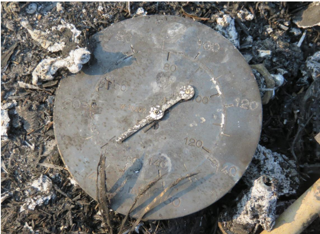
Figure 13: The airspeed indicator as it was found on site, indicating a speed of approximately 100 kt / 54 mph
