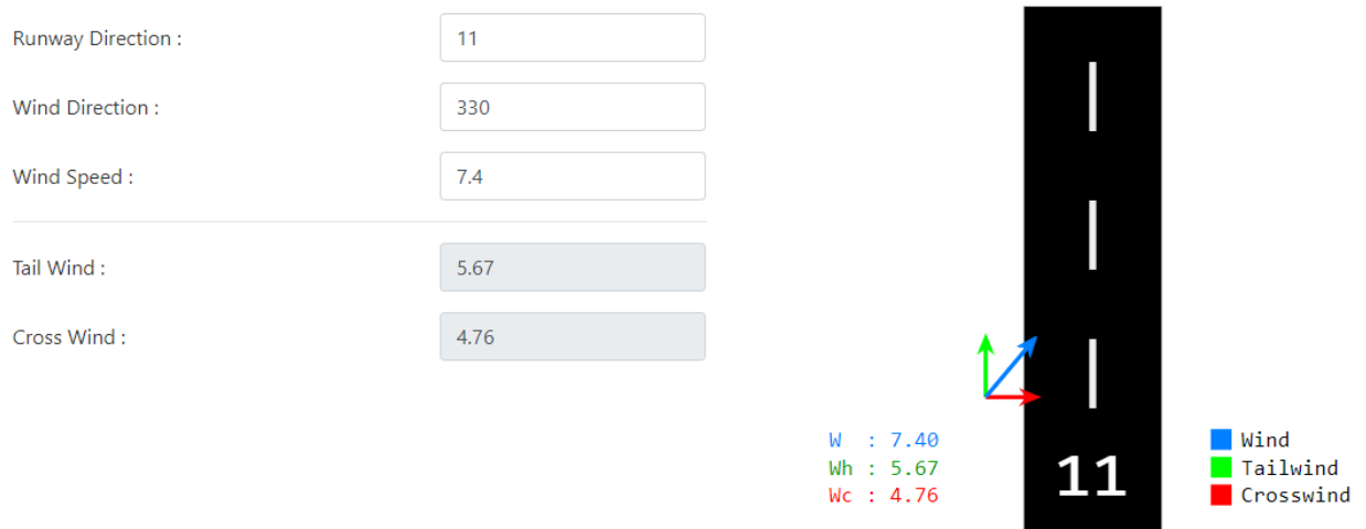
Figure 18: Schematic of the prevailing winds at the time of the accident flight
