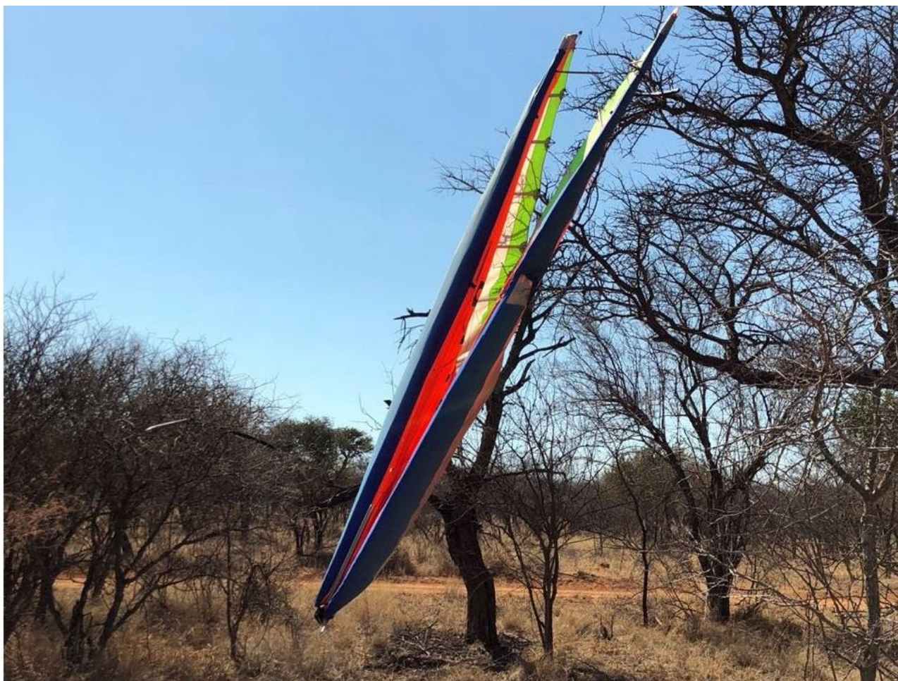
Figure 4: The wing came to rest on a tree after separating from the body of the microlight.
