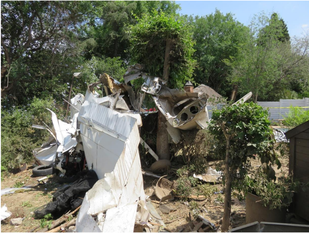
Figure 11: The aircraft fuselage broke in half after impacting a tree
