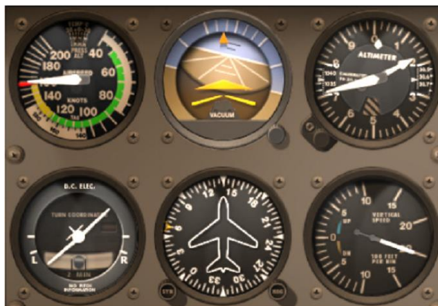
Figure 12: An example of the instrument panel of an aircraft in a spiral dive (Source: http://www.studyflight.com/spiral/ )
