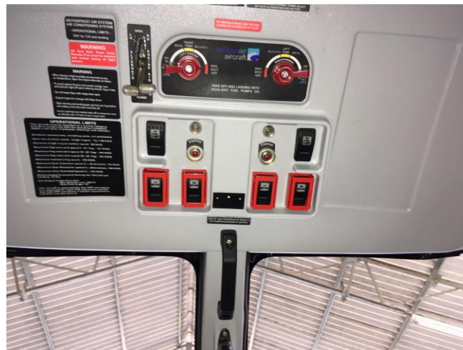
Figure 20: Fuel control selectors for the aircraft (Vulcanair) used by the pilot during conversion.
