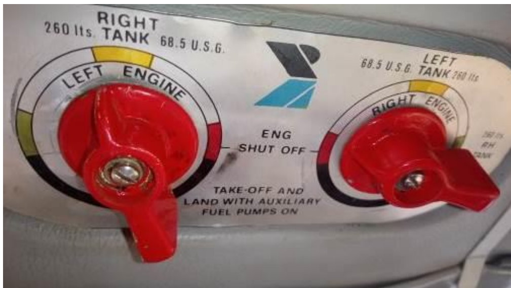
Figure 4: Positon of the fuel valve selectors as found at the accident site.
