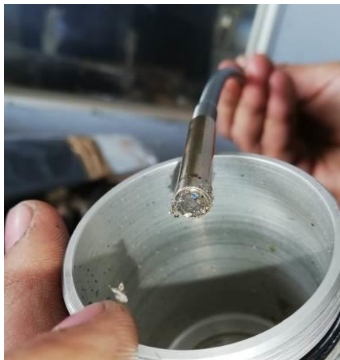
Figure 18: Debris and metal filings.
