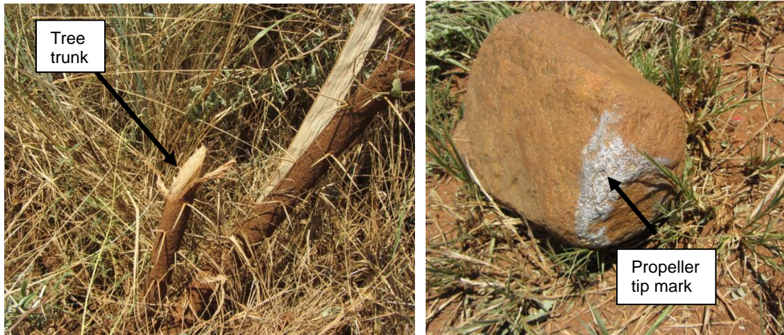
Figure 6 & 7: A small tree trunk severed by the left-hand propeller and a small rock with propeller tip marks.
