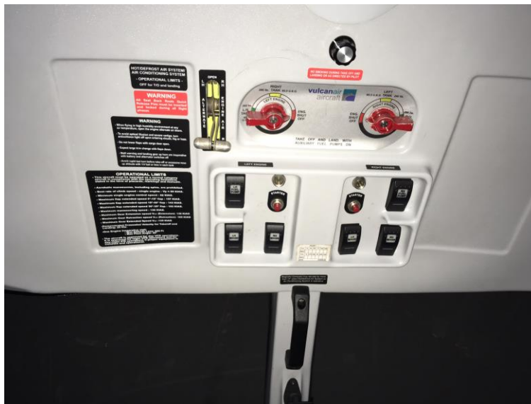
Figure 19: The flight simulator fuel control selectors.
