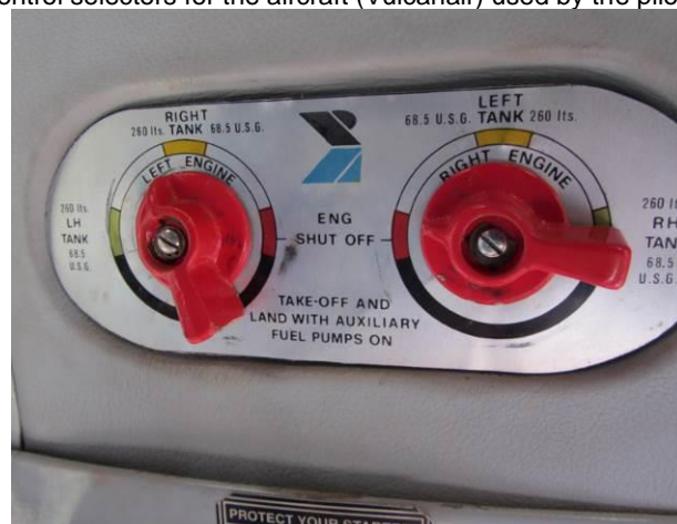
Figure 21: Accident aircraft fuel control selectors.
