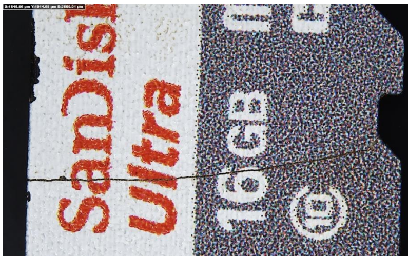
Figure 4: The damaged micro SD card with a crack in the middle.
