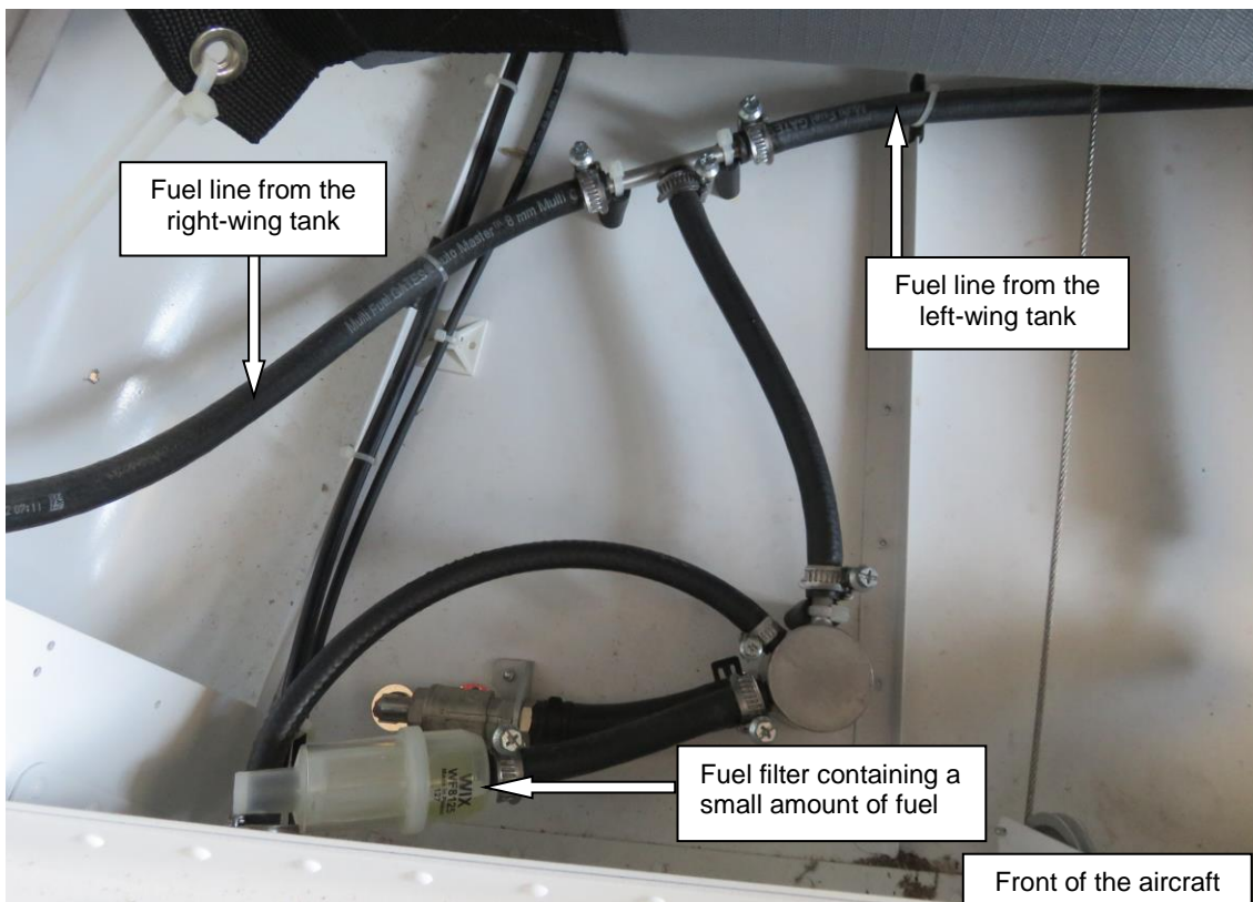
Figure 4: Fuel lines from the left- and right-wing tanks feeding under gravity into a T-fitting (this fuel plumbing is installed behind the two seats)
