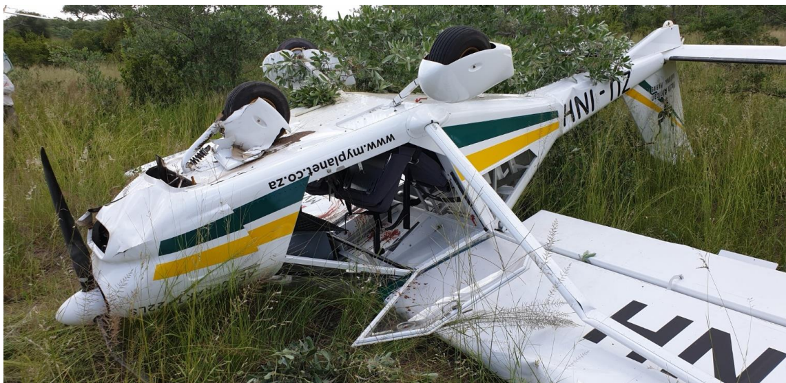
Figure 1: The aircraft as it came to rest in an inverted position.
