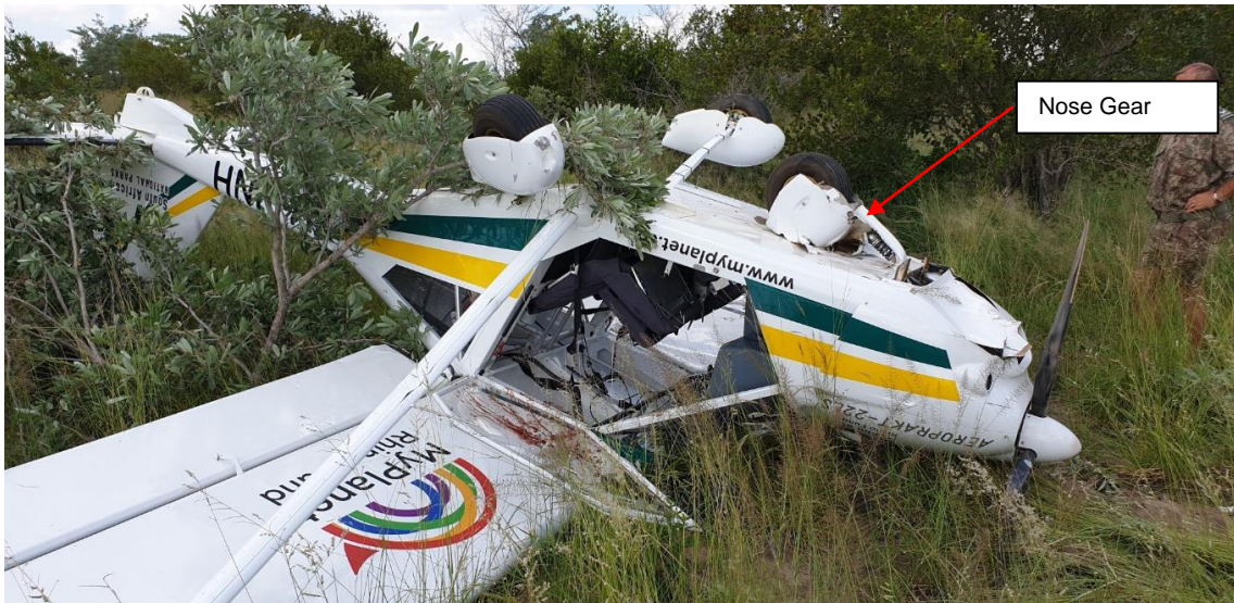
Figure 2: The nose gear could be seen bent backwards
