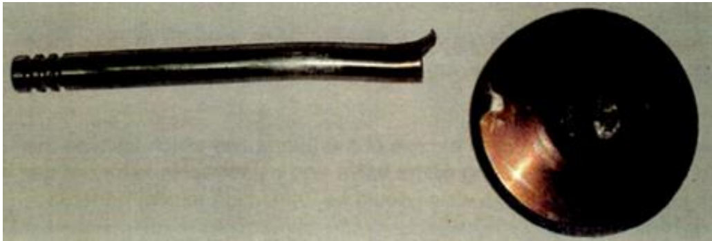
Figure 5: Showing the failed valve on number 4 cylinder
