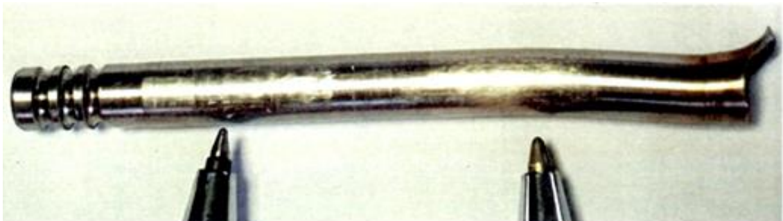
Figure 6: Shows the wear on the failed valve stem on cylinder number 4
