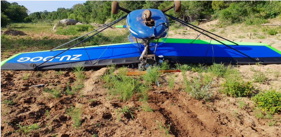
Figure 3: Ground marks showing that the nose wheel dug in before the aircraft nosed over (Photograph courtesy of the ATO)
