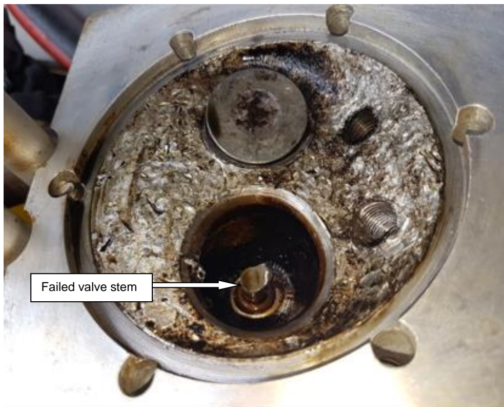
Figure 4: The failed valve stem on number 4 cylinder (Photograph courtesy of AMO)
