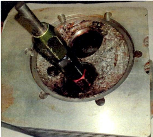
Above Picture The No go gauge showing same size on the Other side of the Exhaust valve
