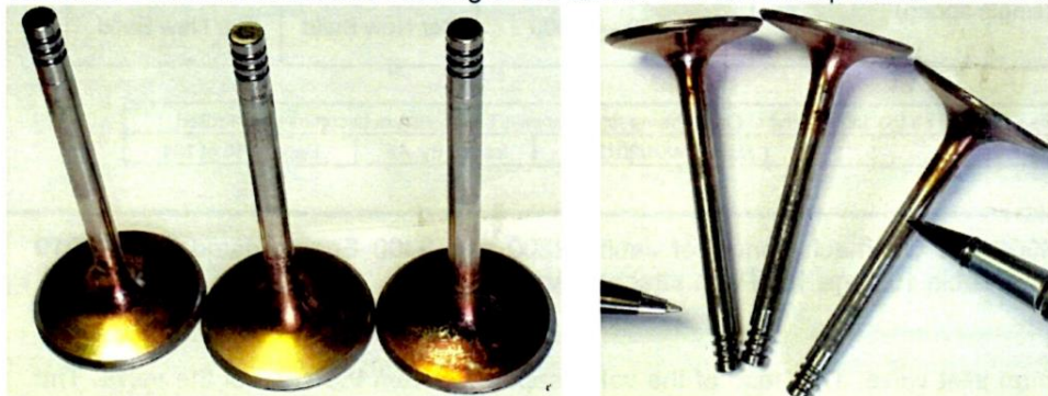
Above pictures showing the condition of the other valves and on the right showing the wear markings on the valves
