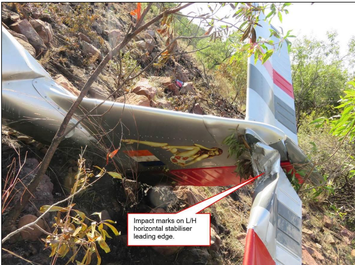
Figure 6: A view of the tail section taken from the left-hand side showing the impact marks on the leading edge.
