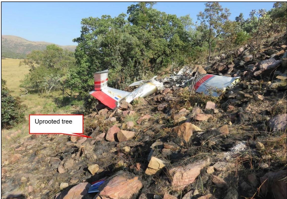
Figure 5: A view of the wreckage taken from the right-hand side showing the uprooted tree.
