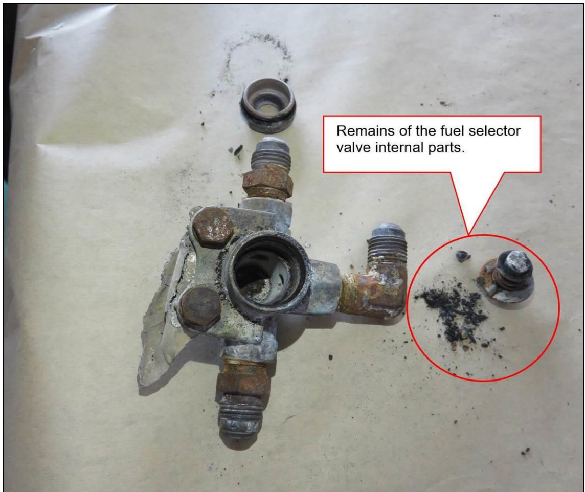
Figure 10: A fuel selector valve after it was disassembled at an approved AMO.
