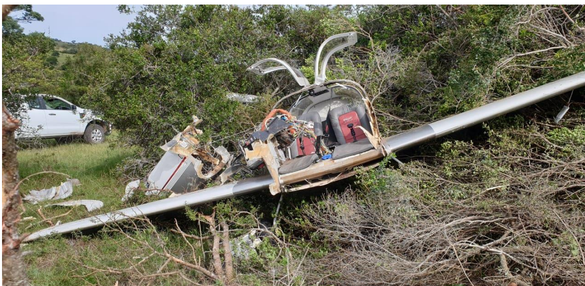
Figure 2: Front view of the damage sustained by the aircraft. (Picture: Rob Williamson)
