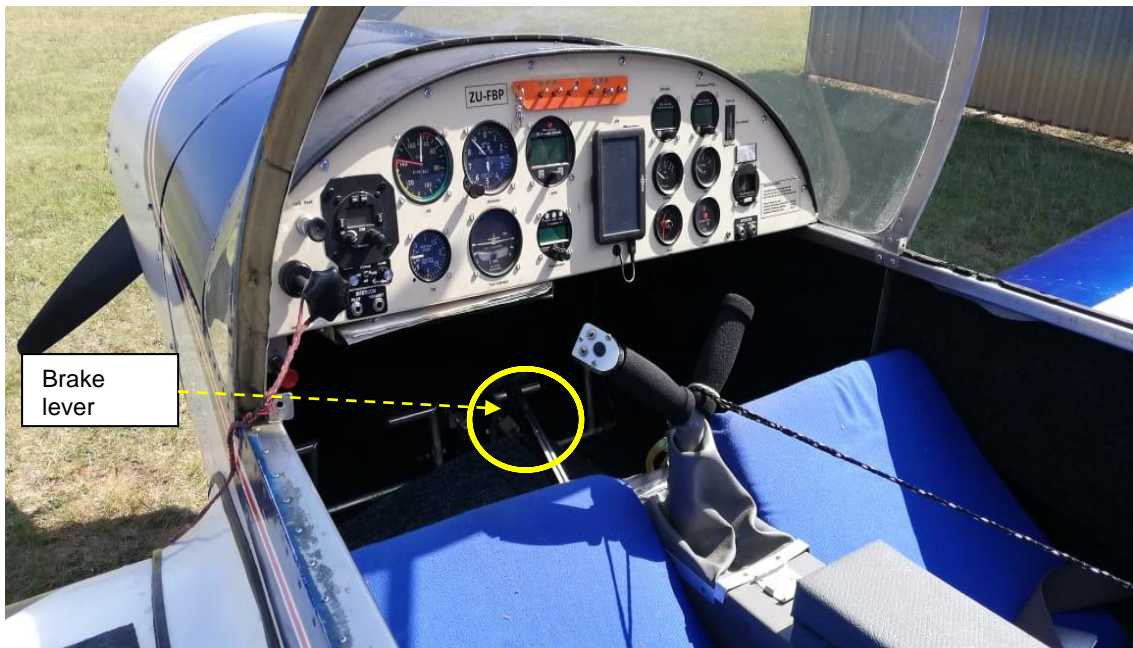
Figure 3: The aircraft's cockpit area with the rope secured from the control stick to the elevator.
