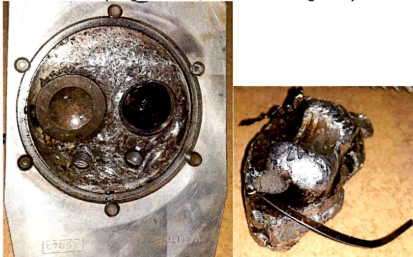
Photo 5: Exhaust valve seat, piston- and head conditions (digital)
