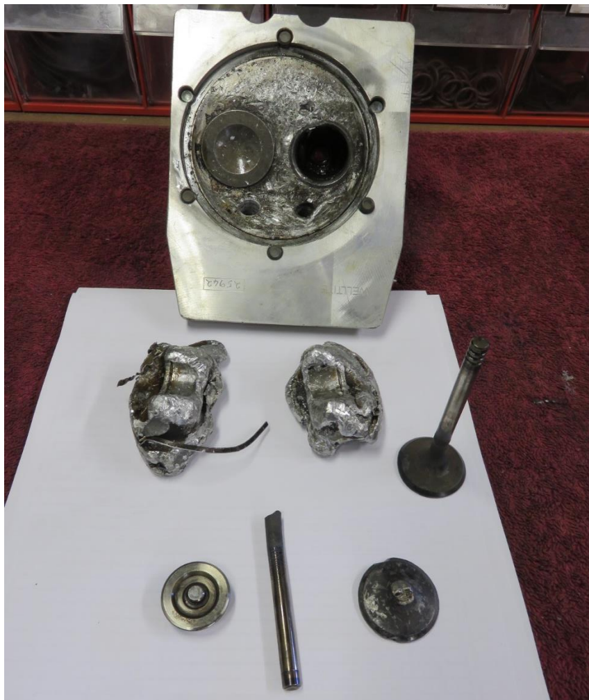
Figure 7: The 3 pieces of the fracture exhaust valve (bottom) and a used valve (right side)
