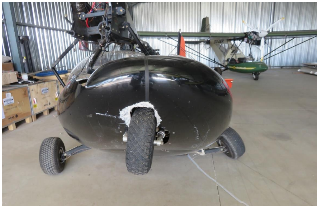
Figure 3: The front view of the aircraft with the boom structure bent to the right (post recovery)
