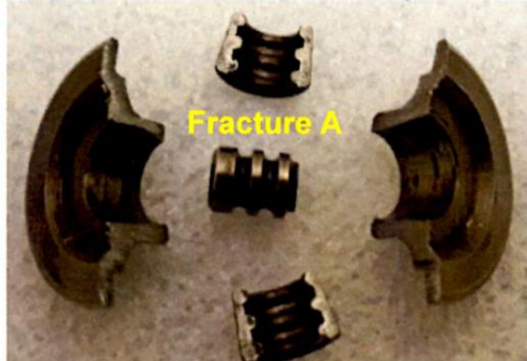
Photo 6: Position of fracture A, top valve spring washer condition (digital)
