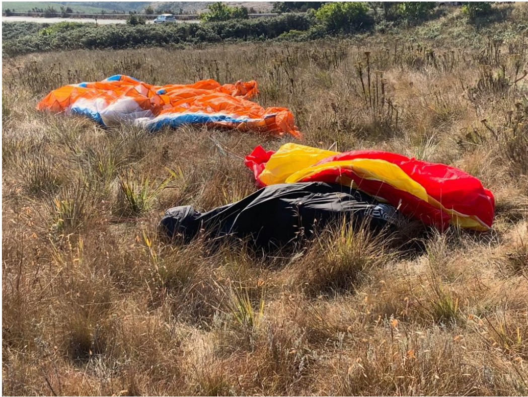
Figure 5: A harness, paraglider and reserve parachute which were not fully deployed. (Source: SAHPA)
