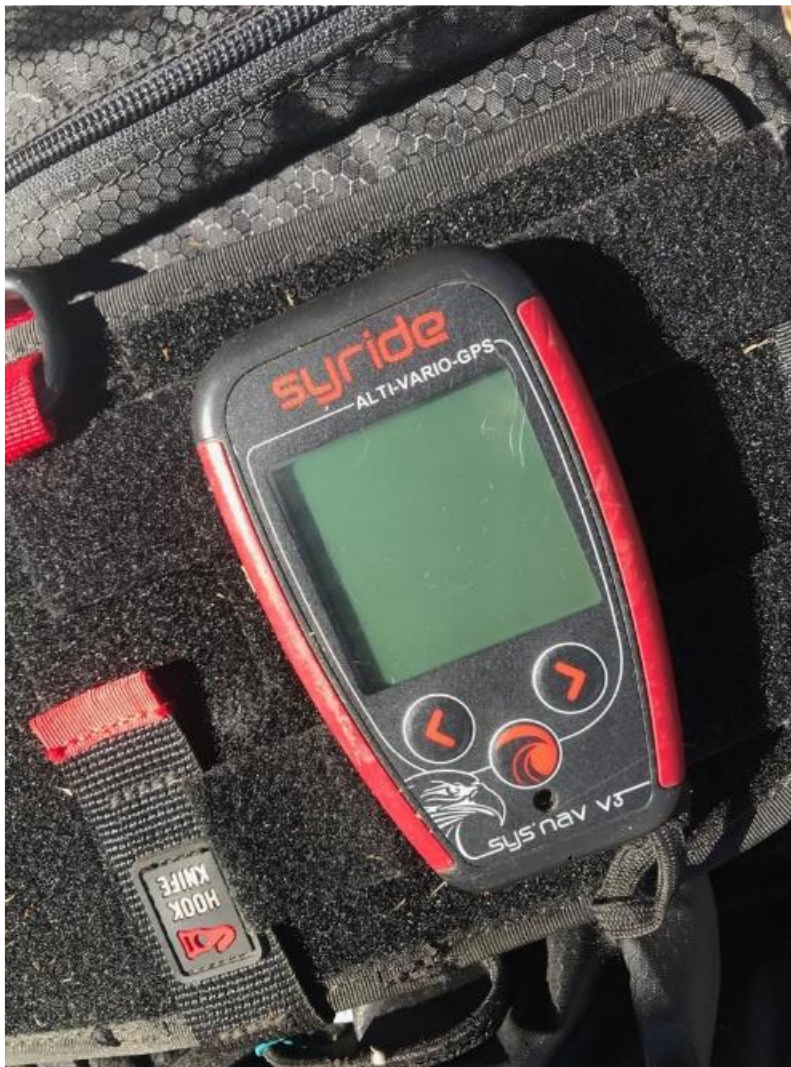
Figure 7: The Variometer instrument. (Source: SAHPA)
