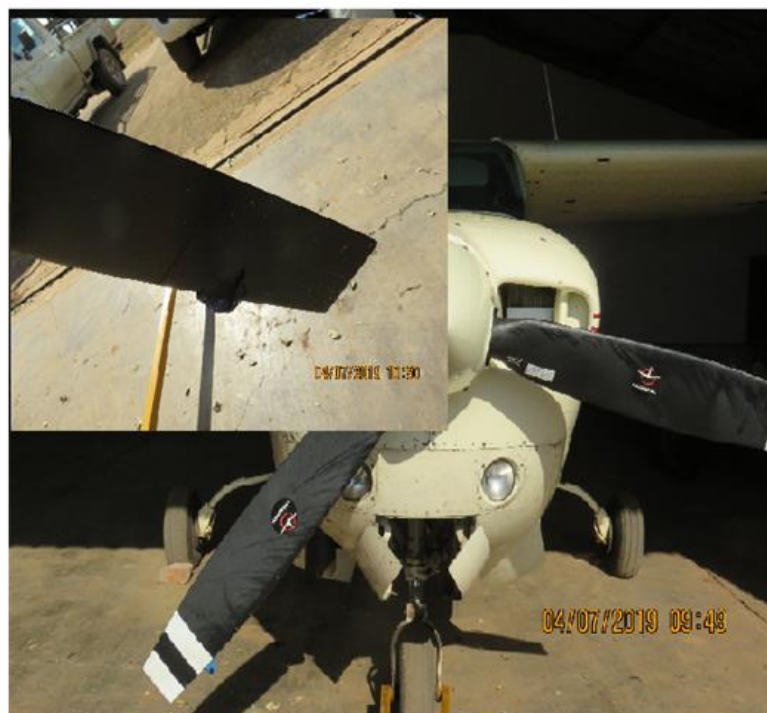
Figure 4: The front view of the propeller with white stripes has better visibility when spinning. The inset shows the rear of the propeller with no white stripes, which makes it invisible when spinning.
