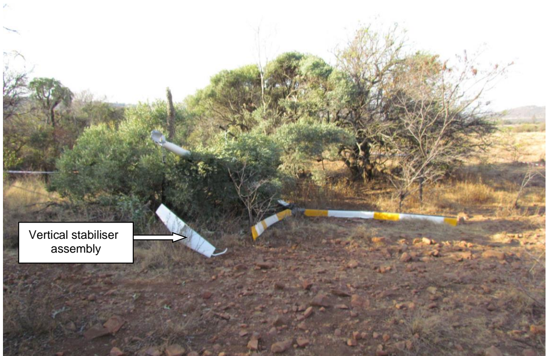
Figure 3: The vertical stabiliser assembly that broke off was found lying below the tail boom.
