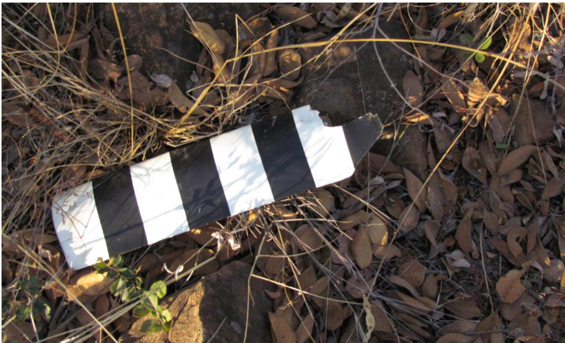
Figure 7: One of the fractured tail rotor blades that was located on-site.
