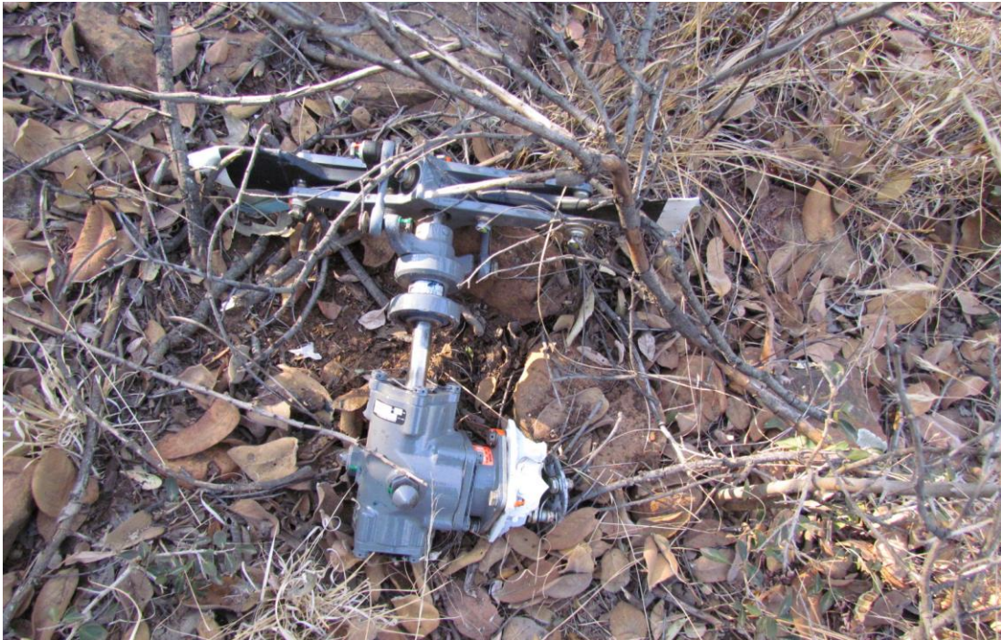
Figure 8: The tail rotor gearbox and hub assembly as they were found on-site.
