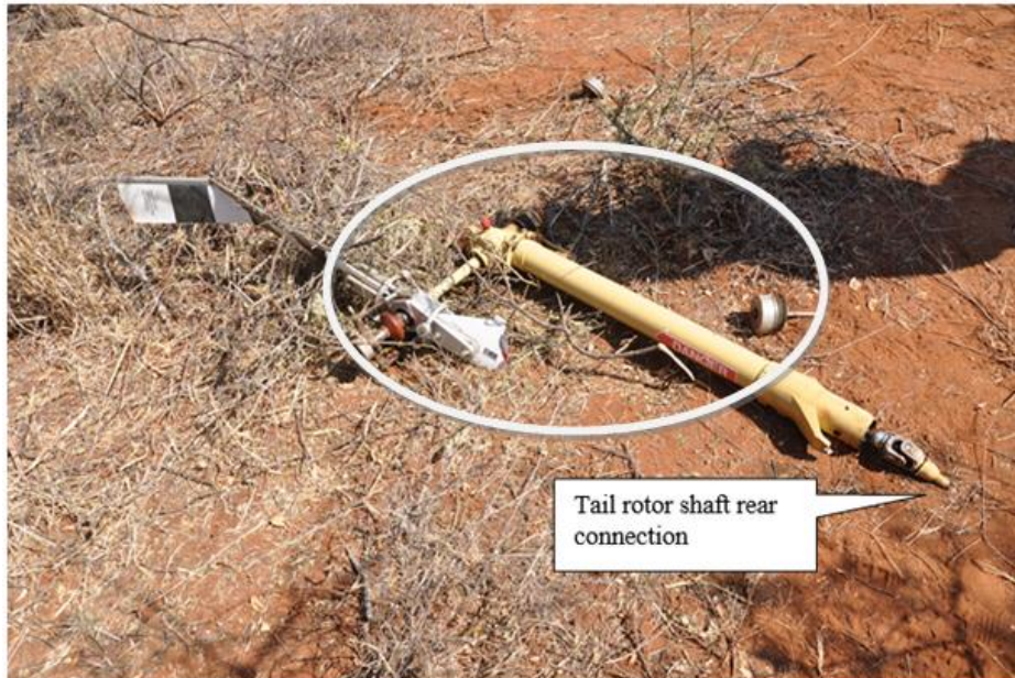
Figure 10: The rear tail rotor drive shaft.
