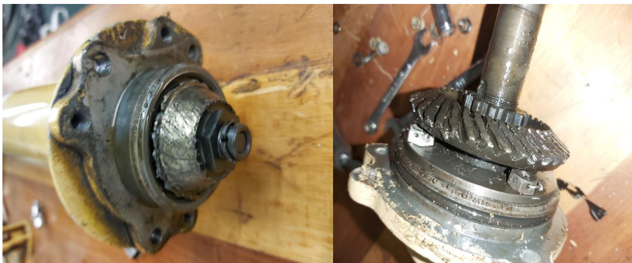
Figure 13 & 14: A closer look at the worn pinion gear teeth and worn bevel gear teeth.
