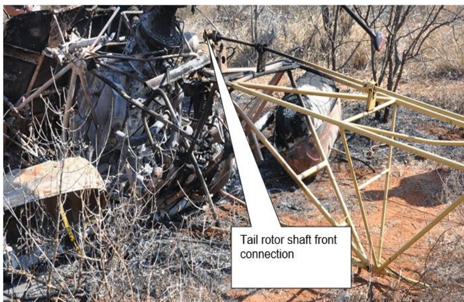
Figure 9: The front tail rotor drive shaft.
