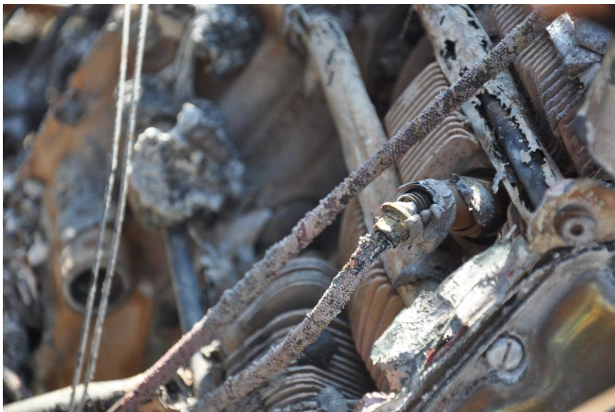
Figure 8: Engine wiring destroyed by post-impact fire.
