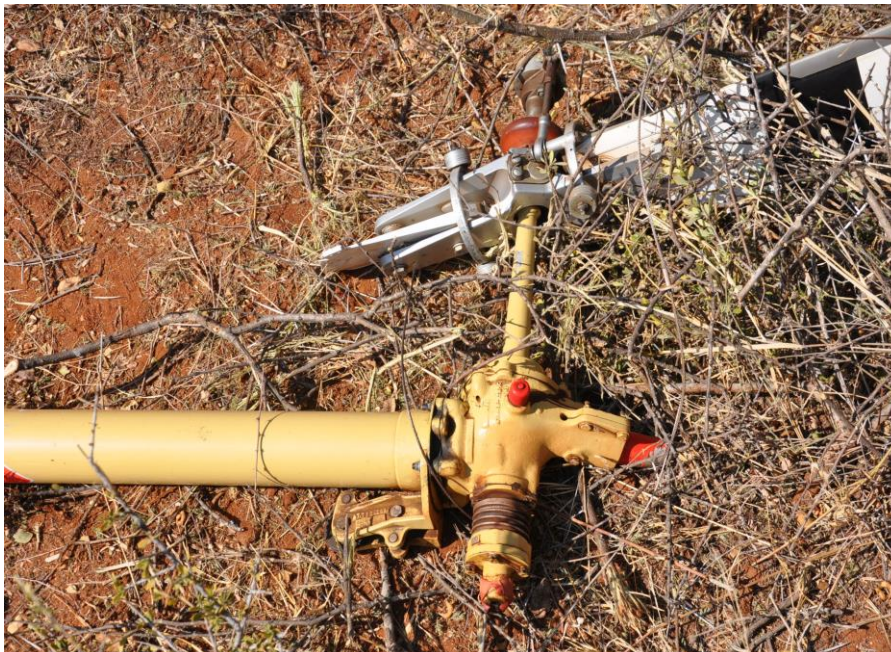
Figure 11: The tail rotor gearbox as it was found on-site.
