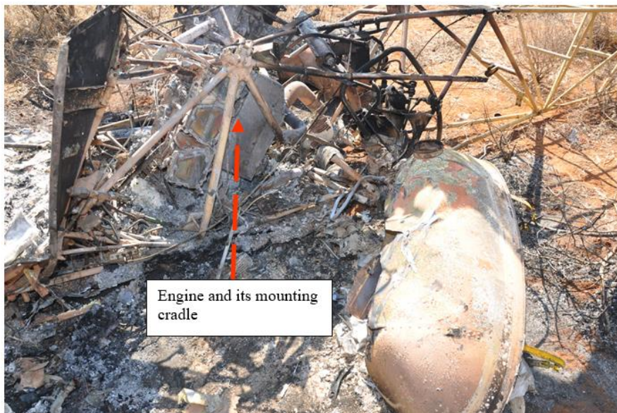
Figure 7: Burnt engine post-accident.
