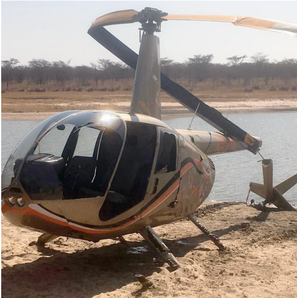
Figure 3: The helicopter after recovery with damage to the main rotor system and tail rotor system.
