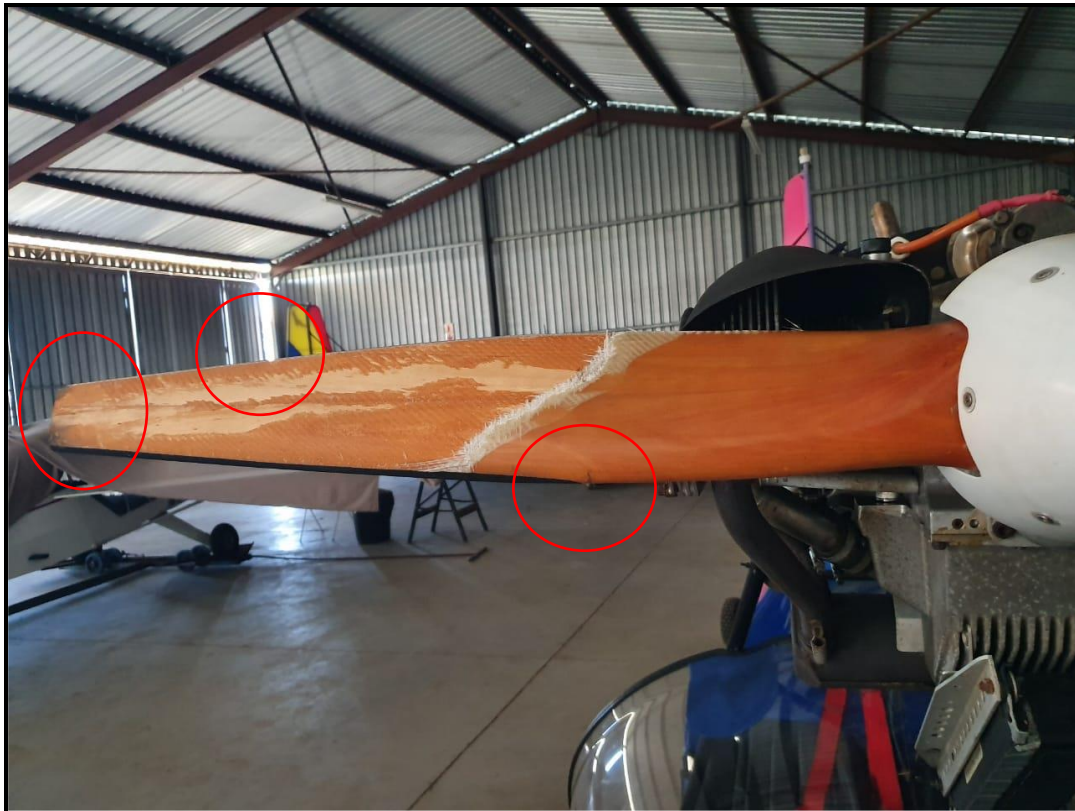
Figure 2: Damage on the propeller blade.
