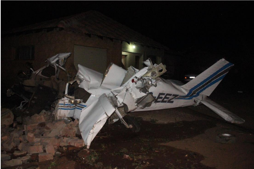
Figure 16: The wreckage and fuel and water spillage after the accident. (source: SAPS)
