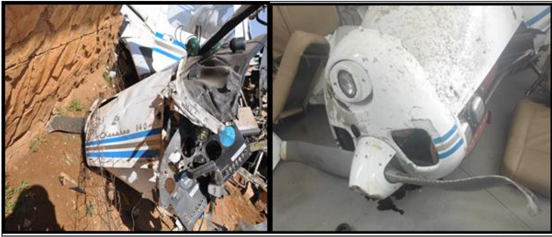
Figures 12 and 13 The aircraft and the propeller blade with the blade tips curled forward, indicative of a high-power setting.
