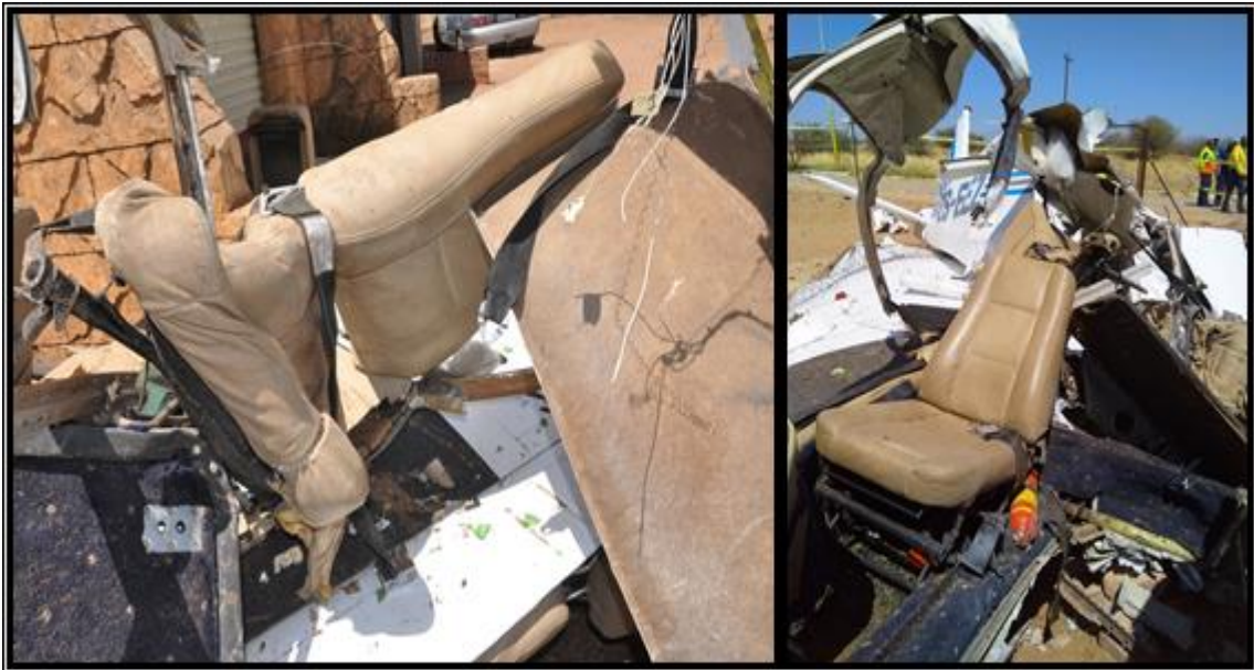
Figures 14 and 15: The damaged pilot seat (left) and the passenger seat (right).
