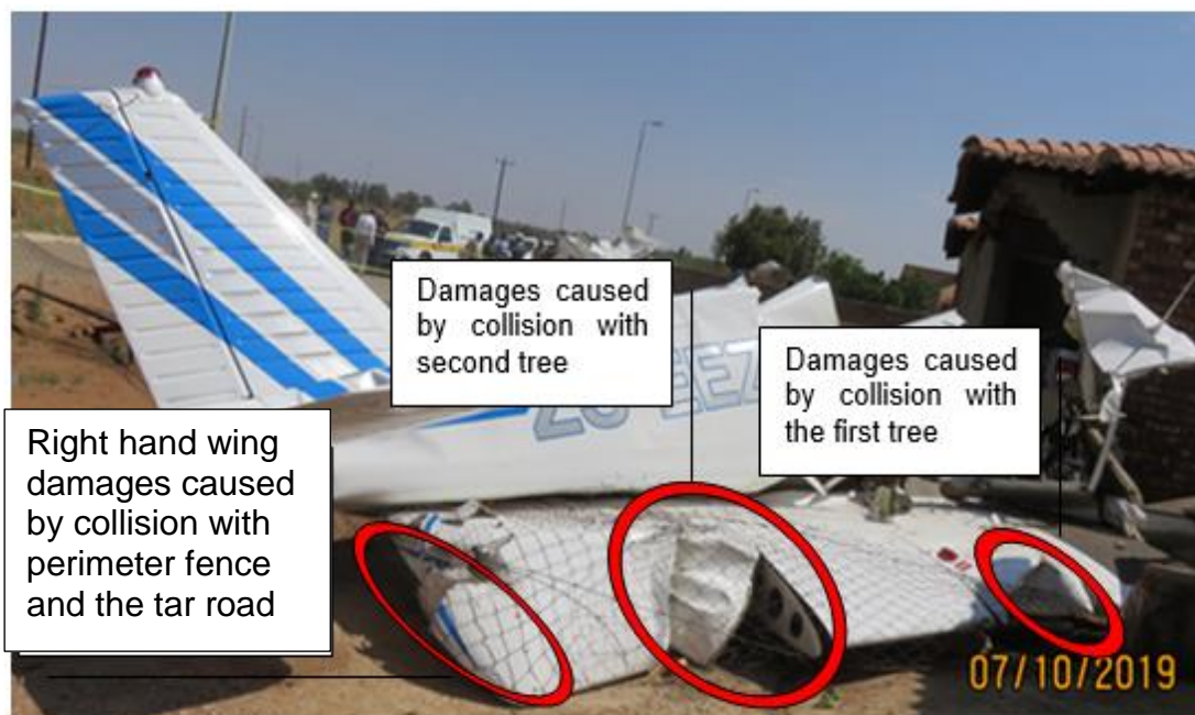
Figure 11: Damages on the right-wing leading edge and wing-tip.
