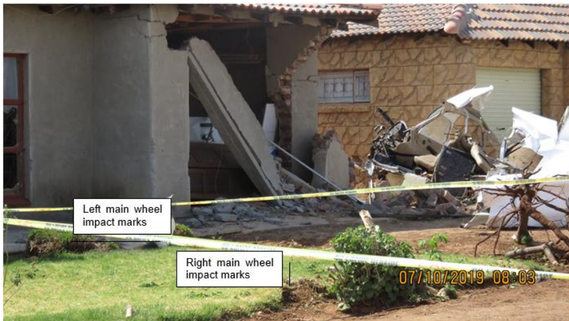
Figure 10: The impact points show the initial direction (southerly) of the aircraft before impacting the house. After impact, the aircraft turned left and came to a stop, facing north east.
