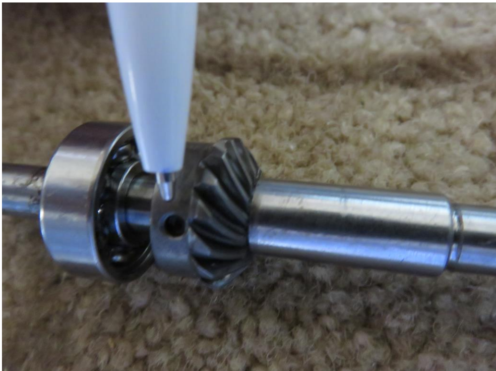
Figure 3: Picture of the lock pin hole.
