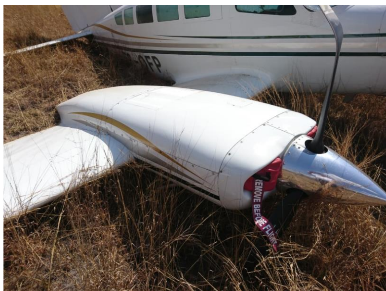
Figure 6: View of the damaged propeller following the collapse of the right-hand main landing gear.
