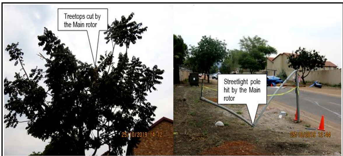
Figure 7: Damage caused by the main rotor strike on both the tree and streetlight pole.
