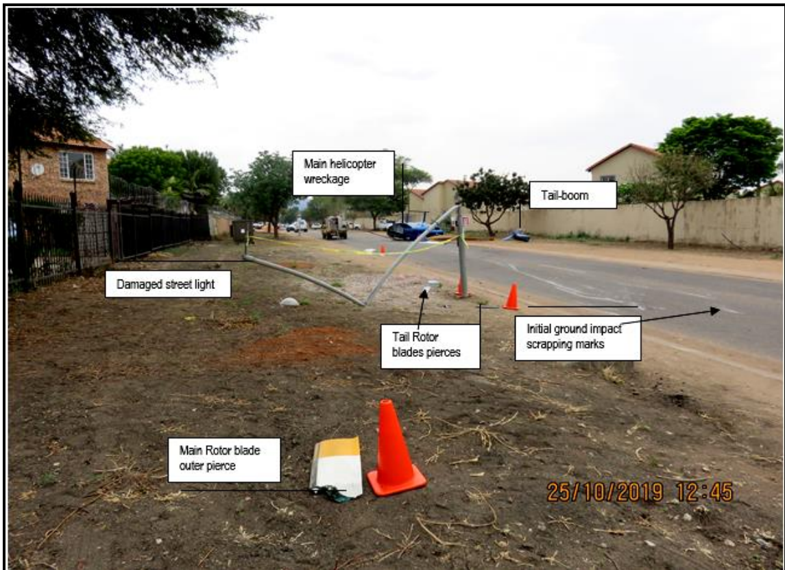
Figure 8: The wreckage distribution as it was observed at the accident site.
