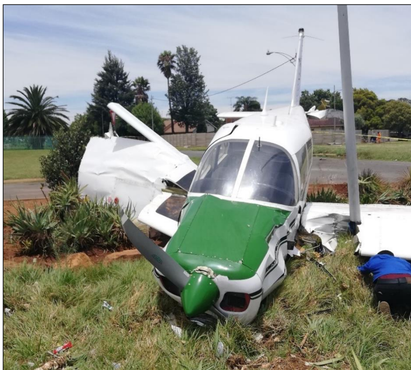
Figure 2: Aircraft damage following the accident sequence.
