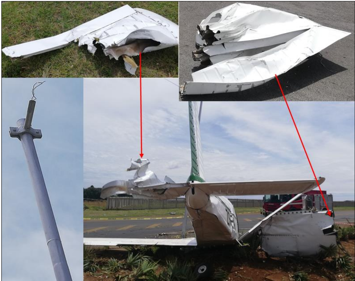
Figure 5: The first lamp pole the aircraft collided with (bottom left), debris of the left-side elevator (top left), debris of the outboard right-side wing (top right), and the aircraft wreckage (bottom right).
