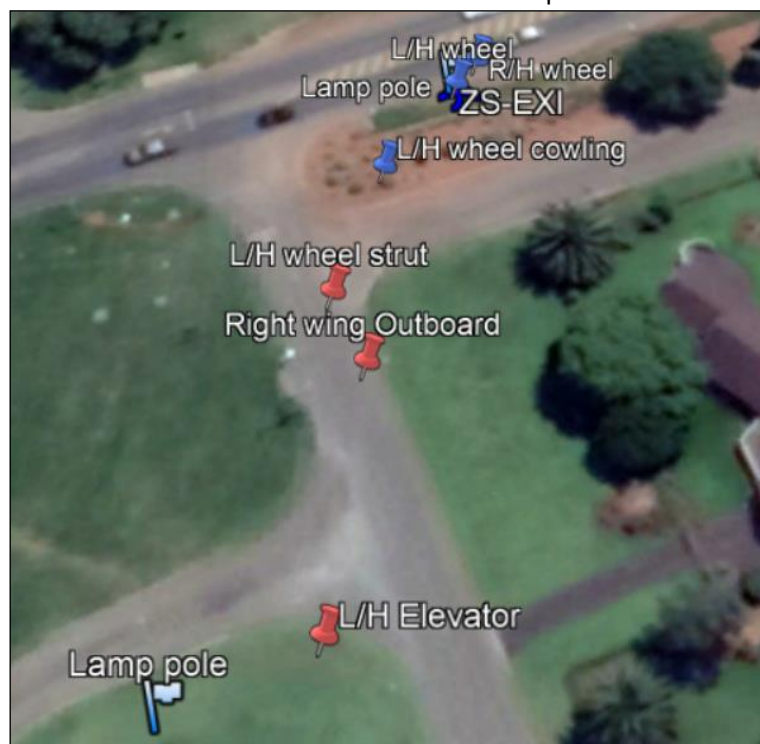
Figure 4: Location of components found at the accident site.
