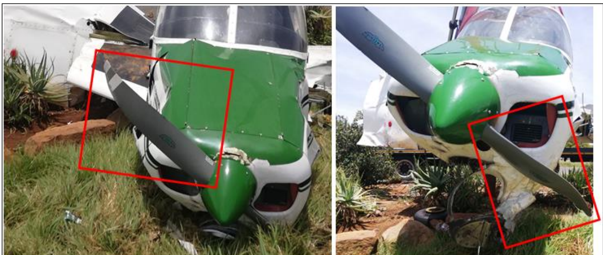
Figure 8: (Left) Propeller blade bent backwards. (Right) Propeller blade bent forwards.
