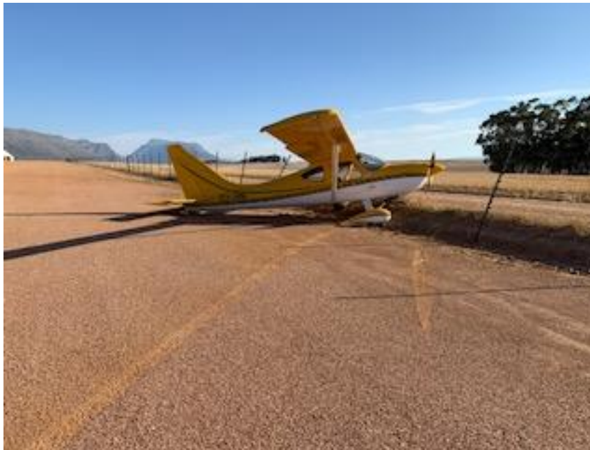
Figure 2: Starboard view and the ground scars leading to the perimeter fence. (Source: Pilot)
