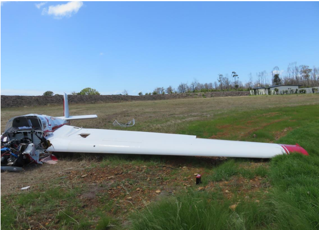
Figure 11: A view of the left wing, which displayed substantially less damage than the right wing.
