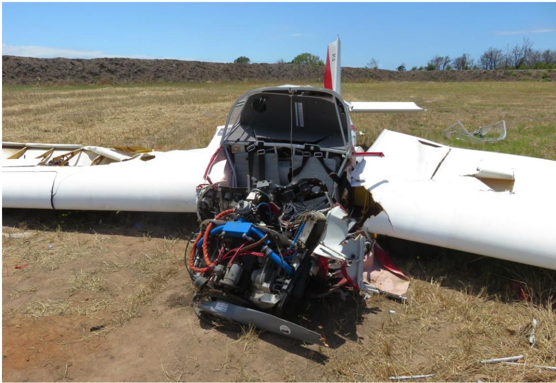
Figure 10: Close-up view with one of the propeller blades destroyed up to the hub assembly.
