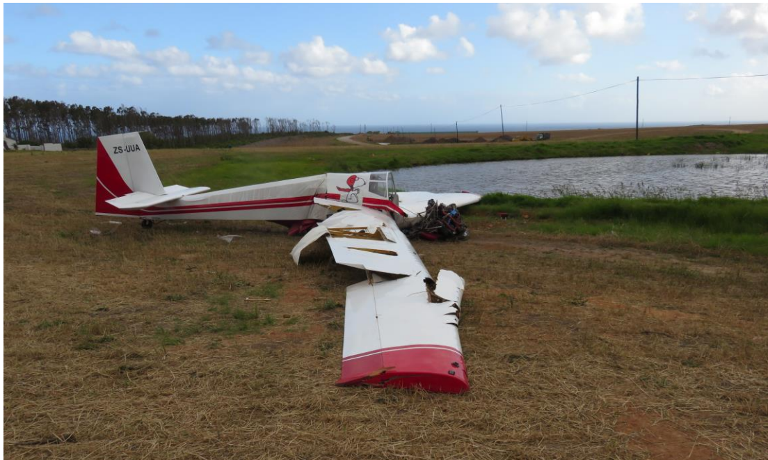
Figure 12: A view of the right wing, which displayed substantially more damage than the left wing.
