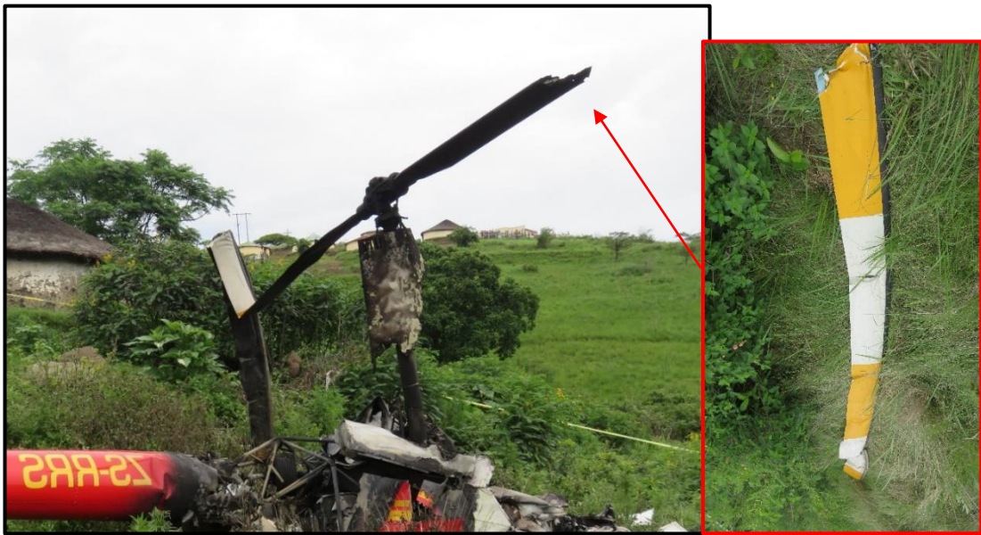
Figure 6: The main rotor blade assembly after the accident.
