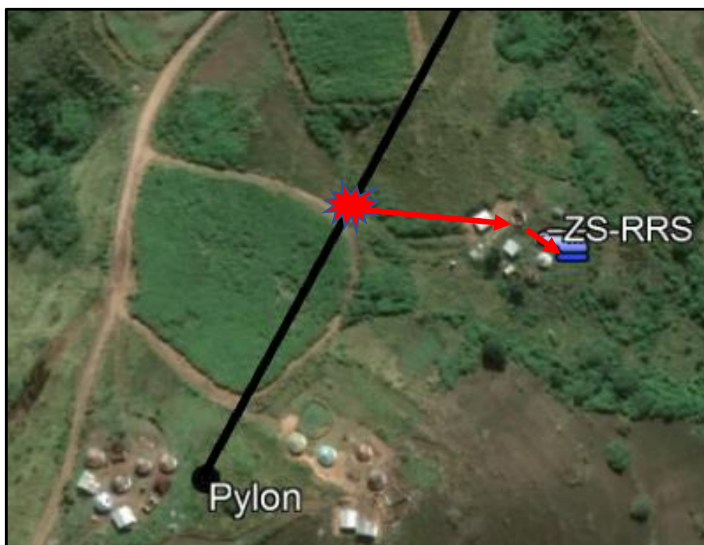
Figure 5: The flight path of the helicopter's impact with powerlines and, later, the ground. (Source: Google Earth)
