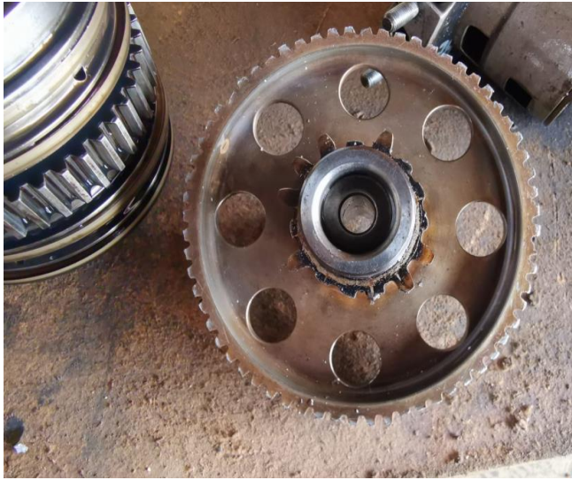
Figures 6 & 7: The missing gear teeth on the impeller intermediate drive (left) and a failed impeller bearing (right).
