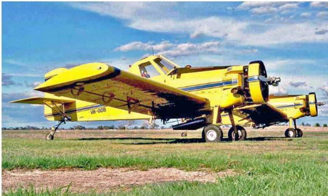
Ayres AT-301 Air Tractors VH-ODB and VH-ODM at Tintinara SA in May 1989 Designed by Leland P. Snow, the AT-302 designation indicates 320 gallon hopper and P&W R-1340 radial engine
