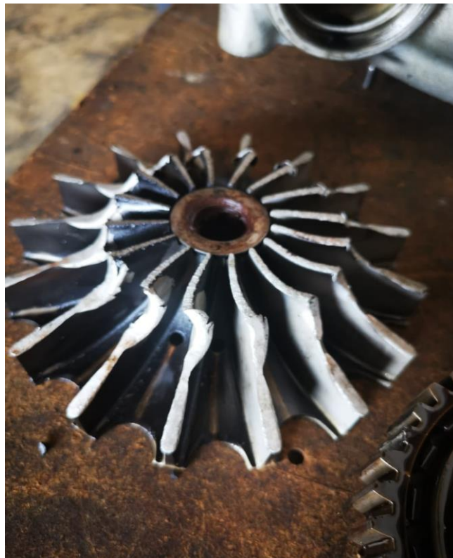
Figure 8: The damaged impeller.
