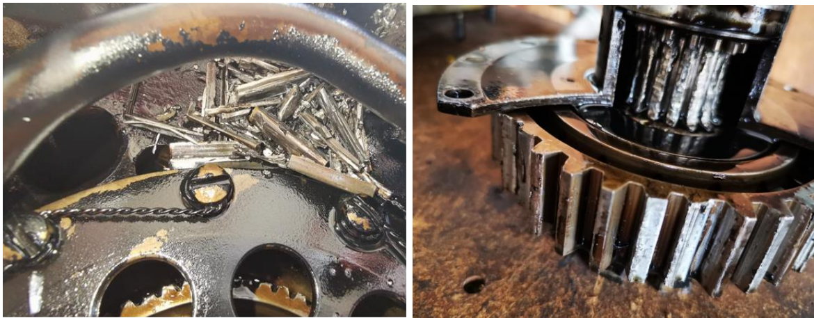
Figure 9 & 10: The gear teeth shavings (left) and the impeller drive shaft with missing gear teeth (right).
