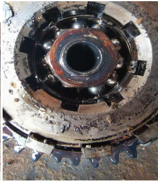
Figures 6 & 7: The missing gear teeth on the impeller intermediate drive (left) and a failed impeller bearing (right).
