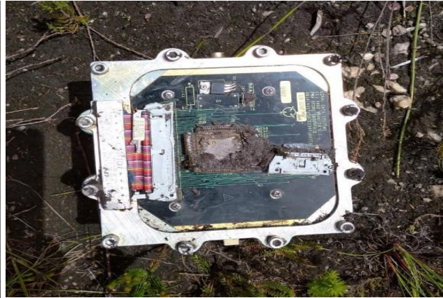
Figure 8: ZS-CAR - Recorder opening &amp; read-out - BEA - 3rd Feb 2020
