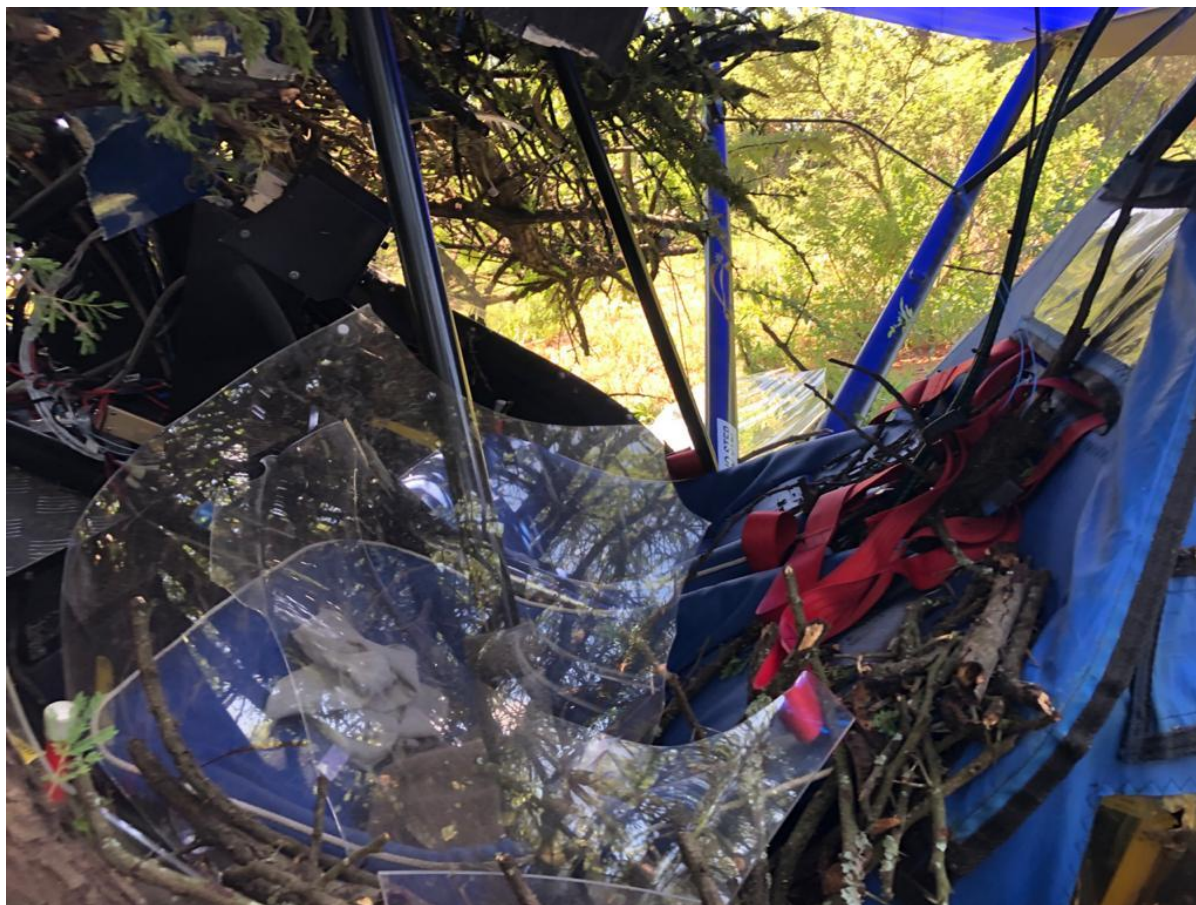
Figure 6: The cockpit cage and safety harnesses after the accident. (Source: Insurance assessor)
