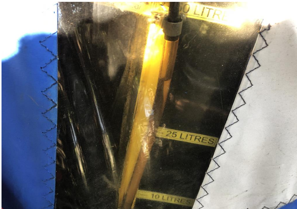
Figure 4: Fuel gauge showing the amount of fuel remaining in the tank. (Source: Insurance assessor)
