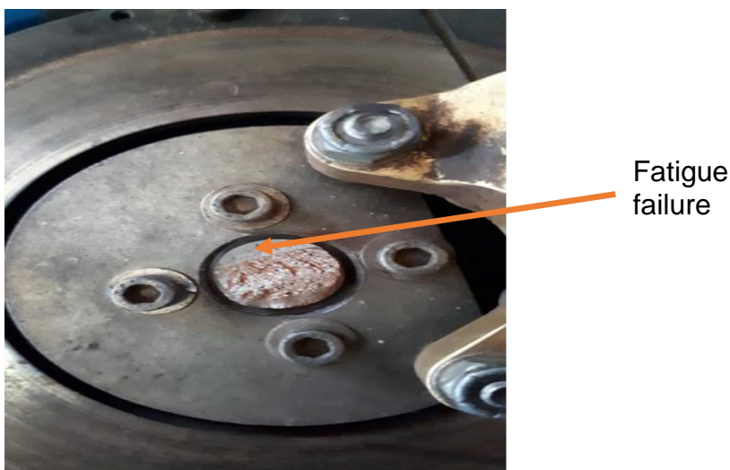
Figure 2: Pre-crack condition on the in-board wheel bearing area. (Source: AP)
